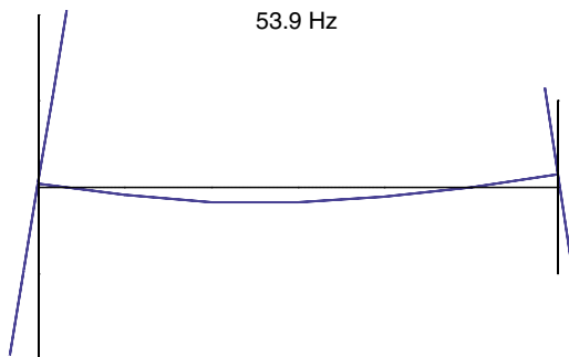
Figure A.7 H-shaped aluminium structure mode 1
