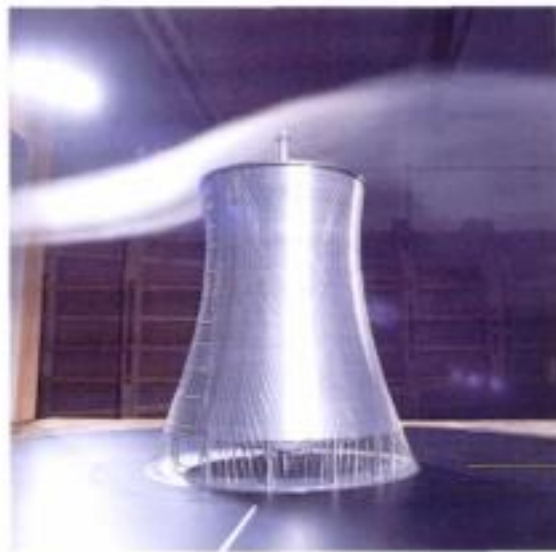
5.106 A model of the Schmehausen cooling tower undergoing testing in the wind tunnel
