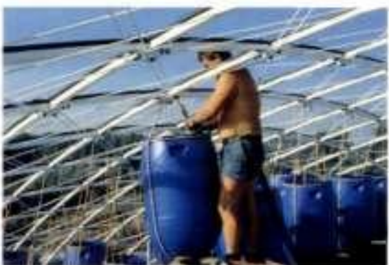
6.20 Water barrels representing partial snow load
