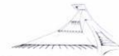
The roof is retracted. Its movements are controlled with the "lasso" cable looped around its lower perimeter
