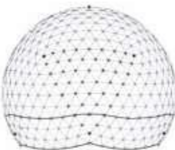
6.3 The geometry of the geodesic dome based on the icosahedron principle
