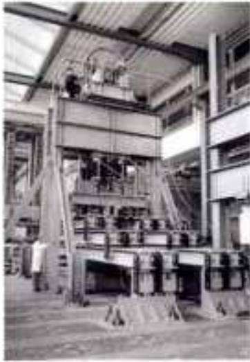
5.47 The cable-saddle fatigue testing machine at the Zurich ETH
