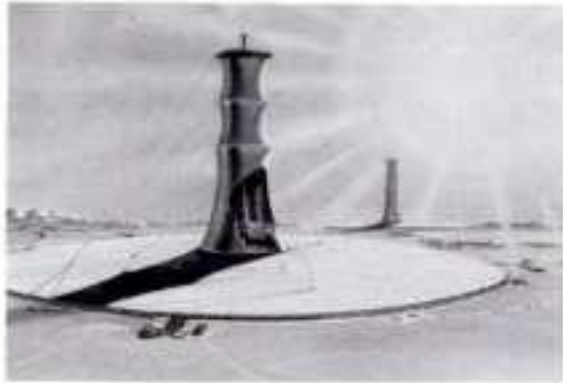
11.41 Drawing of a 100 MW plant with a cable-net or membrane skin chimney
