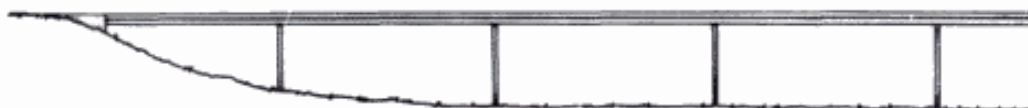
8.92 Shorter spans make it possible to reduce the depth of the deck, permitting the use of open sections, while flexible steel columns eliminate the need for bearings
