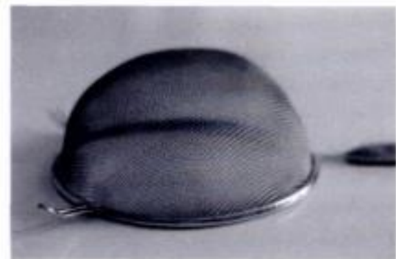
A wire kitchen sieve, a hemisphere formed from a flat sheet of square mesh provides a useful demonstration of the principle
