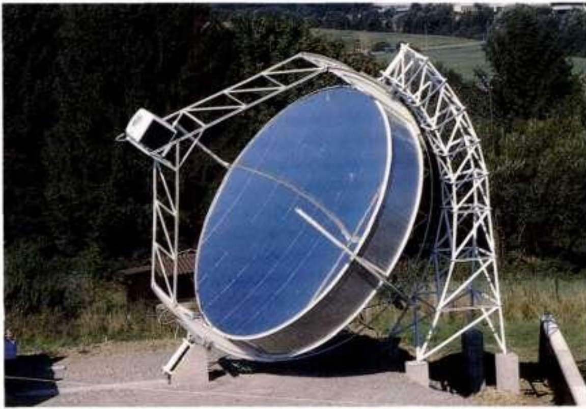
11.36 The first complete 7.5 m-system with Stirling engine and generator installed at Stuttgart 1989
