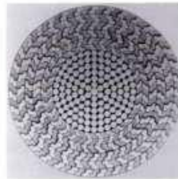
5.26 Section through a locked-coil rope
