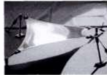
By mechanically applying forces from the edges of an open surface a plane steel sheet assumes a saddle shape
