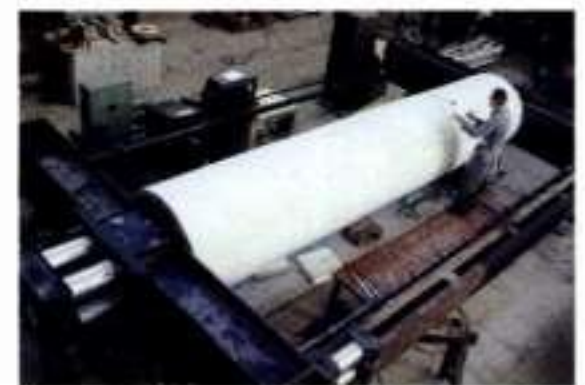
3.16 Tests on concrete tubes under axial force and bending at the Otto-Graf-Institut, University of Stuttgart
