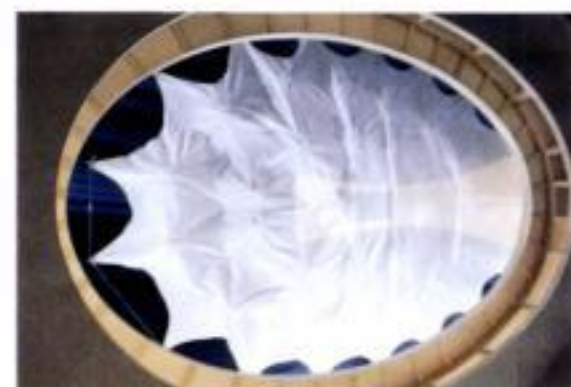
7.13-7.16 The kinematic model of the Montreal Stadium showing stages in the extension of the roof (view from below)
