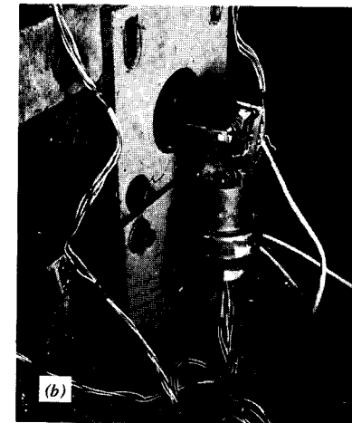
Fig. B.12 Rotation gages: (a) mechanical; (b) electrical.
