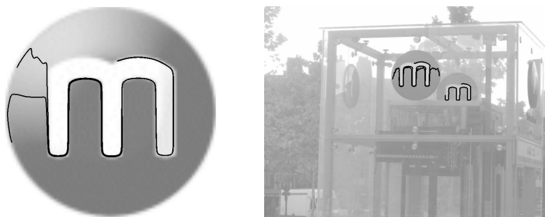
Fig. 10. The logo on the left is searched for in the image on the right, using a similarity invariant encoding. There are 9 matches, and none of them is false, in the sense that they correspond to the same pieces of the logo. The smallest NFA has a value of 4.4 \times 10^{-12} .
