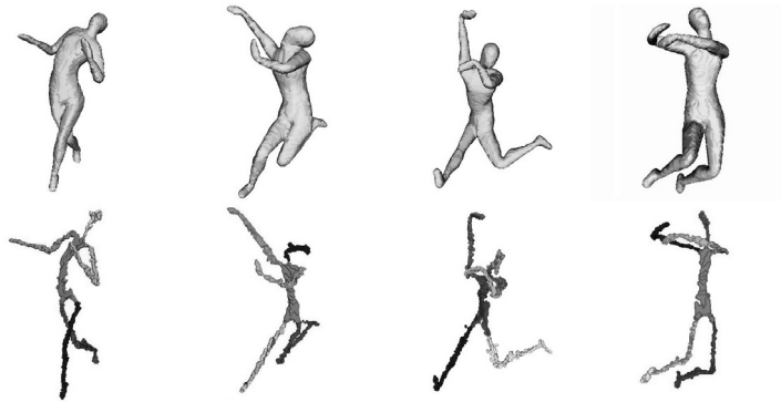
Fig. 7. Medial axes for different exemplars of a 3D human object model, obtained using the average outward flux based thinning algorithm [22, 9]. The medial axis is automatically partitioned into distinct parts, using the labeling technique of Malandain et al. [13].
