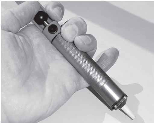
FIGURE 5.26 Priming the desolder pump by pressing down the charger.
