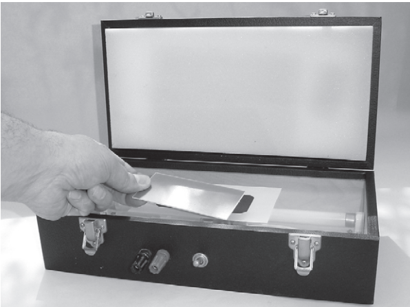
FIGURE 4.30 Placing the LaserStar film and photographic resist-coated printed circuit board into an ultra-violet light box, ready for exposure.
