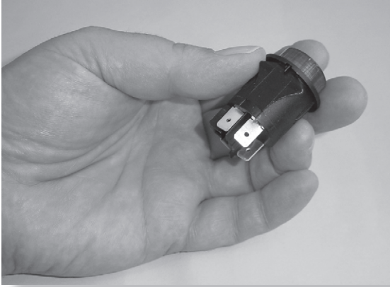
FIGURE 3.47 A mains switch with an integral neon bulb (this particular switch is used in the Bench Power Supply project in Chapter 8).
