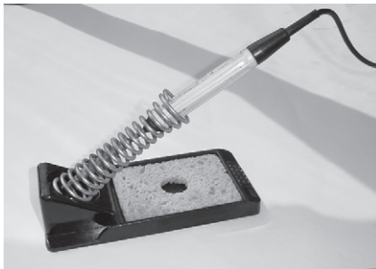
FIGURE 5.28 Use a soldering iron stand when not actually using your soldering iron. Keep the safety risks to a minimum.
