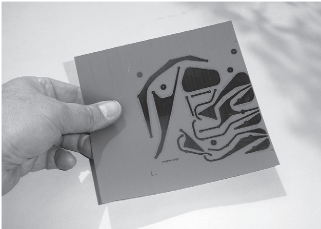
FIGURE 4.31 Lay the Press-n-Peel sheet over the plain copper surface of the copper-clad board.
