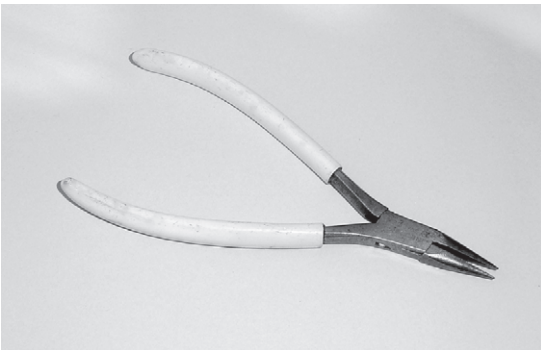
FIGURE 2.15 Miniature long-nosed pliers are extremely useful tools to keep in your electronics toolbox.
