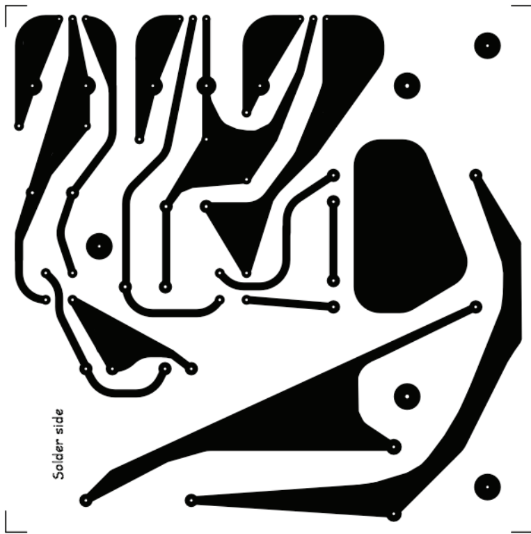
FIGURE 8.27 Bench Power Supply printed circuit board copper track foil pattern (actual size).
