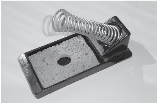
FIGURE 2.9 A soldering iron stand. This particular stand features a sponge.
