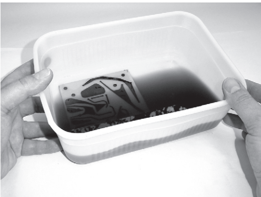
FIGURE 4.35 A makeshift etchant bath — an old ice-cream container, in which the etchant is manually agitated by rocking the tray gently. A good excuse to have some ice-cream!
