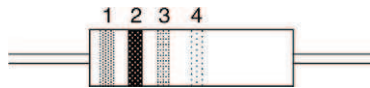
FIGURE 3.11 A resistor showing the four coloured bands that give its value according to the four-band resistor colour code detailed in Table 3.1.
