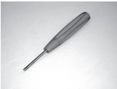
FIGURE 2.23 Terminal pin pusher — just put the pin loosely in place in the printed circuit board, then push home firmly with the pusher.
