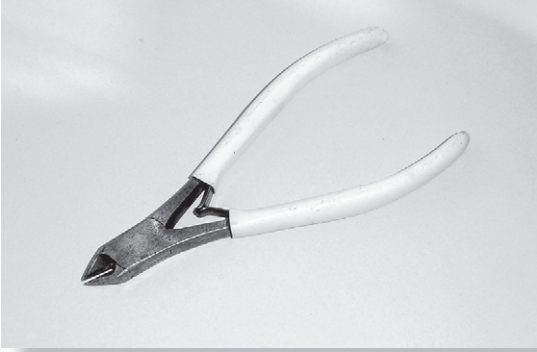
FIGURE 2.14 A good quality pair of miniature side-cutters. After your soldering iron, it's the tool you'll use the most in electronics.
