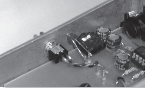
FIGURE 6.22 Simple mounting of a LED to a panel.
