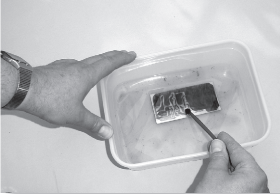
FIGURE 4.24 Developing an exposed, photo-resist coated, copper-clad board.
