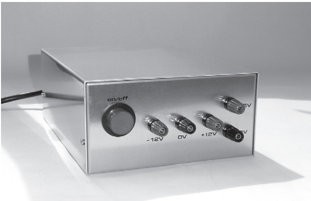
FIGURE 8.20 The Bench Power Supply.
