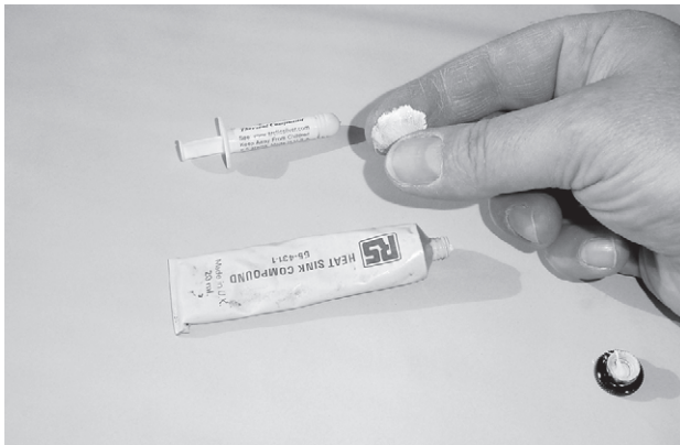
FIGURE 6.26 Thermal compound — supplied in various ways. Put a small amount on your finger and rub between finger and thumb before applying to a component or heatsink surfaces.
