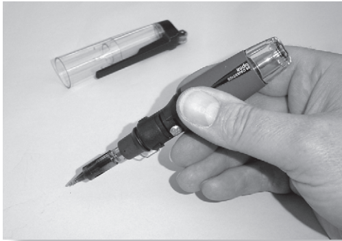
FIGURE 2.3 A gas-powered soldering iron. Small and portable, these can be recharged from lighter fuel butane gas containers.
