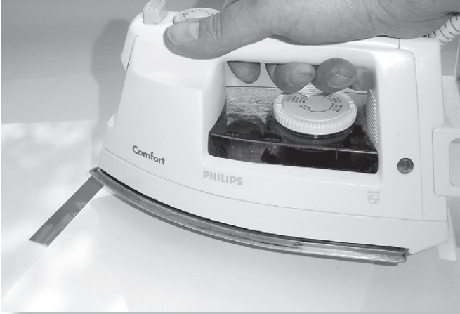
FIGURE 4.32 Using an iron to transfer the image from a printed Press-n-Peel sheet onto the copper surface of plain copper-clad printed circuit board.
