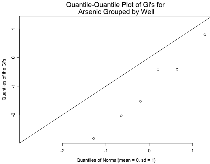
Figure 7.5 Normal Q-Q plot of the normal scores used in the group Shapiro-Wilk goodness-of-fit test for normality of the arsenic concentrations
