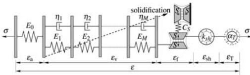
Figure 1. Rheological scheme of the complete hygro-thermo-mechanical model.
