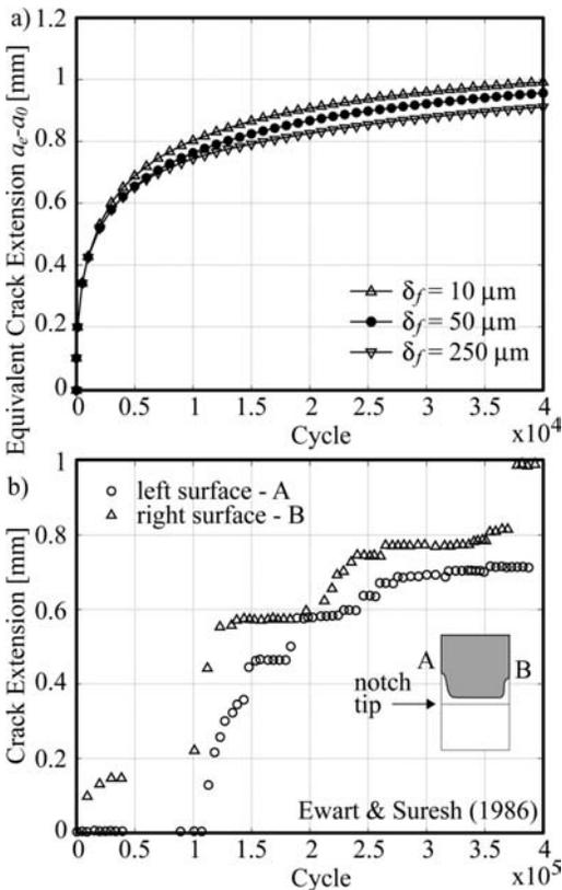
Figure 1. Crack extension a) simulated and b) experimentally observed.
