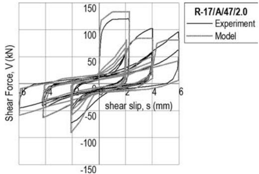
Figure 1. Typical hysteresis loop for specimen. Comparison between experimental results and model predictions.
