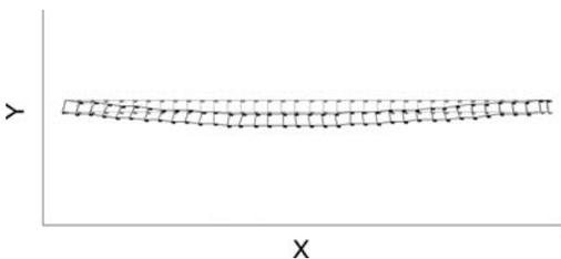
Figure 1. Identified mode shape of Mode 1 (1.67 Hz, 1.4%).
