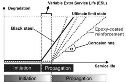
Figure 1. Possible corrosion protection effect of ECR compared to black steel (herein Extra Service Life – ESL).
