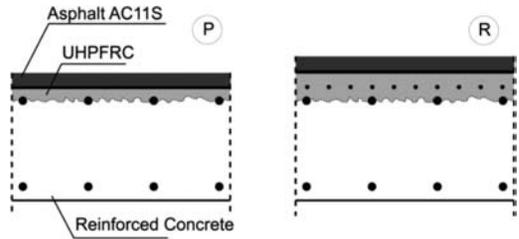
Figure 1. Applications of UHPFRC for protection (P) or as R-UHPFRC for reinforcement (R).
