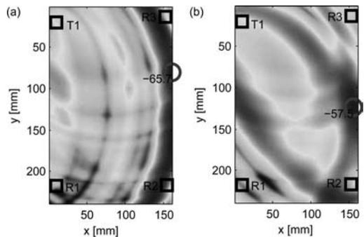
Figure 1. Results of crack detection with the UGW sensor array and the maximum echo. (a) image after 1.101.078 and (b) after 1.399.629 load cycles.
