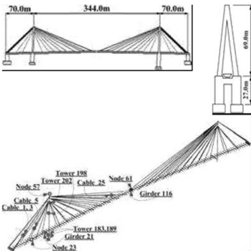
Figure 3. Profile and 3-D model of the Jindo cable-stayed bridge.
