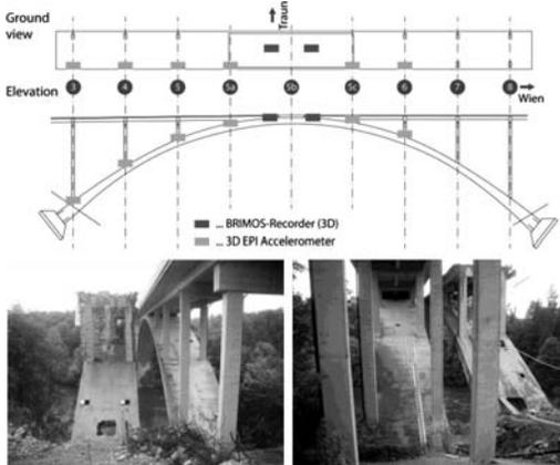
Figure 1. Sensor layout (elevation and ground view) for the dynamic measurement of the arch and photo documentations.
