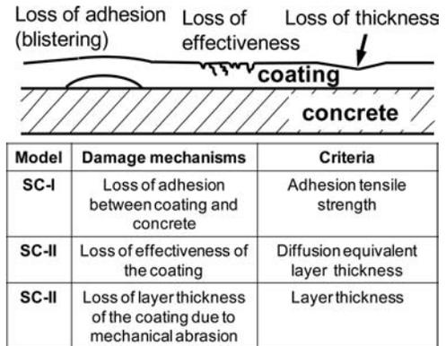
Figure 10. Failure mechanisms of surface coating for concrete.
