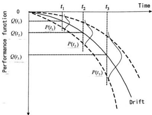
Figure 1. Degrading process of the tunnel lining.
