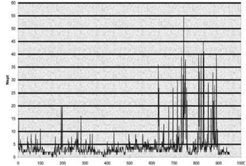
Figure 1. Soil profile at 3 m depth as a function of  $N_{SPT}$ .
