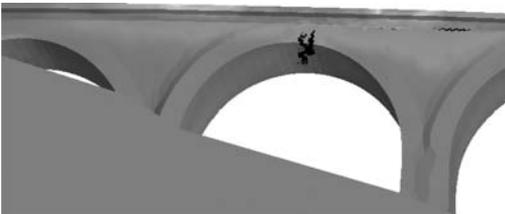
Figure 1. Cracks at the bottom side of a masonry arch bridge.
