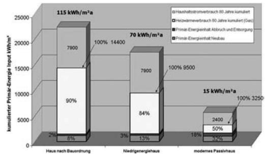
Figure 1. Life-Cycle Assessment comparing standard building stock (according to building code in 2000), low energy standard building and passive house standard building.
