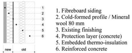
Figure 1. Thermal retrofitting solution – example (Tuca et al. 2011).
