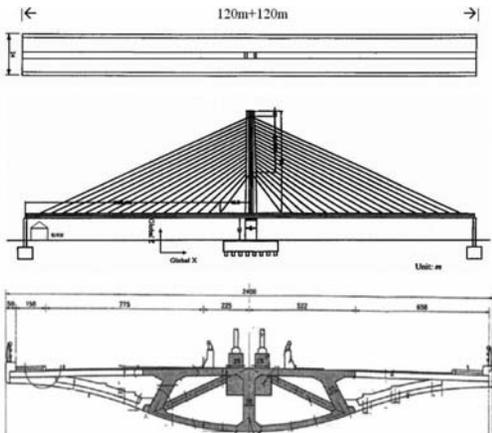
Figure 1. Plan, elevation and cross-section of the Chi Lu Bridge at Nantou Country, Taiwan.
