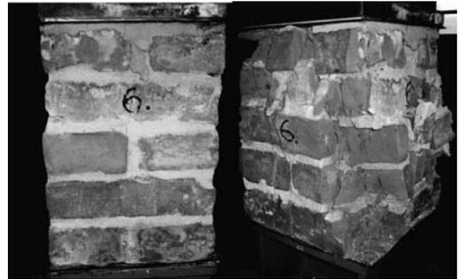
Figure 2. Compression tests on column-type test specimens. Left photo: Crack initiation. Right photo: Failure pattern.
