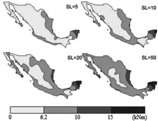
Figure 1. Optimal base bending moment considering aeolian and seismic actions on wind turbines for different structural importance values,  $S_L$ .
