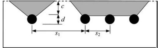
Figure 1. The geometric parameters affecting the spalling (Hunkeler 2006).
