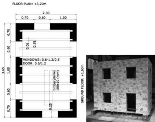
Figure 1. Plan and picture of the two storey building model.
