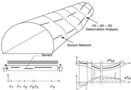
Figure 4. Strain, curvature and deformation analysis (Strauss 2003).
