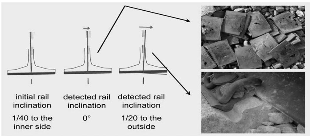
Figure 9. The measuring signal rail inclination allows detecting the condition of the rail pads.
