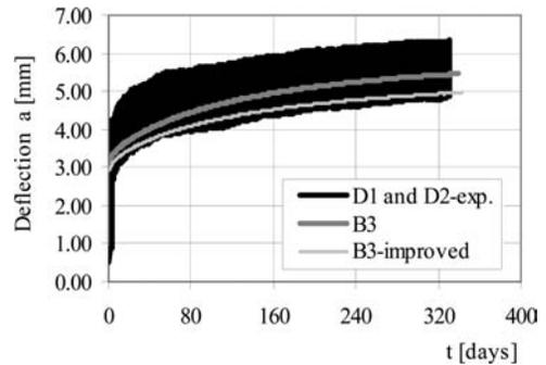
Figure 1. Diagram deflection-time for series D beams concrete class C30/37.
