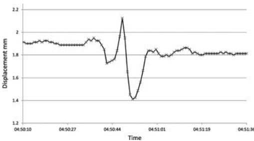
Figure 1. Roller displacement trace showing vehicle passage.
