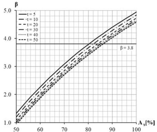
Figure 1. Reliability index  $\beta$  in dependence of shear reinforcement and a reduced remaining service life  $t$ .
