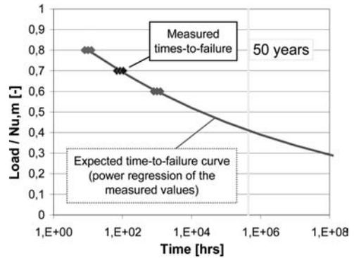
Figure 2. Hypothetical time-to-failure curve with an extrapolation based on a power regression analysis of measured times-to-failure at high load levels.
