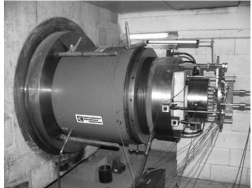
Figure 1. Hydraulic jack with a stay cable anchorage for 43 strands.
