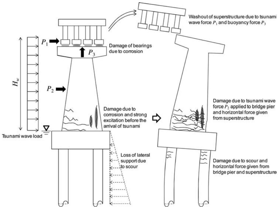
Figure 10. Possible failure mode of bridge under tsunami hazard.
