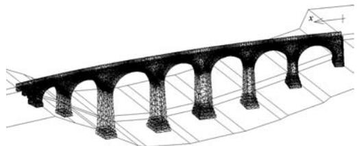
Figure 2. Finite element mesh for a curved bridge (mesh for the soil not shown).
