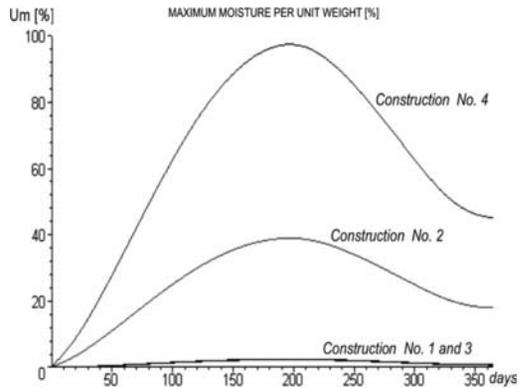
Figure 2. Changes in the values of moisture per unit weight in the most critical spot within the building construction over time.
