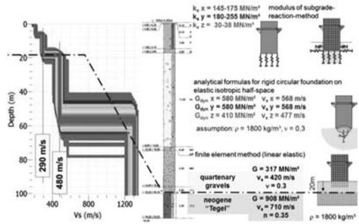
Figure 2. Comparison of the obtained soil-parameters: Results from measuring the Rayleigh-waves and from the soil-structure-interaction.
