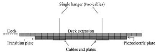
Figure 2. Position of the EH device on the bridge.
