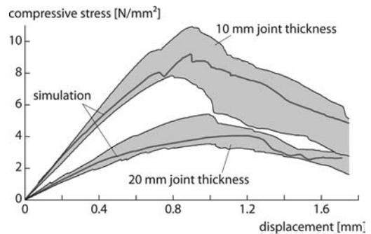
Figure 1. Stress-displacement curves of masonry compressive tests with one mortar joint. Experimental scatter and results from numerical simulations.
