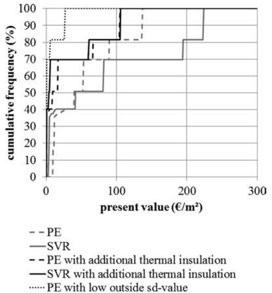
Figure 1. Cumulative frequency of the present value with 10% mvs and a low  $n_{50}$ -value for different flat roof constructions with a building price index of 3% and an interest rate of 4%.
