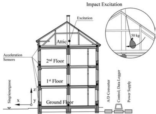
Figure 2. Vertical distribution of the acceleration sensors within test object, and experimental test set-up.
