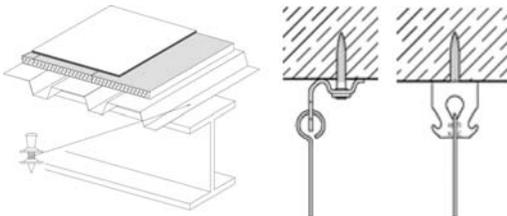
Figure 1. Anchorages with power-actuated fasteners.
