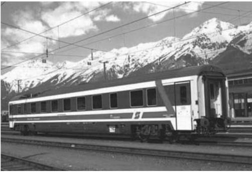
Figure 5. The Permanent Way measuring coach EM 250 is running with a speed of up to 250 km/h.
