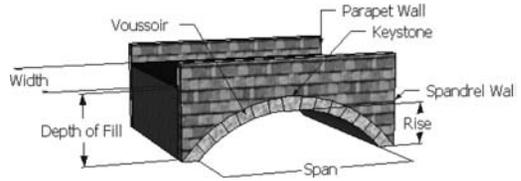
Figure 1. Typical masonry arch.
