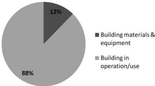
Figure 1. Ecological assessment at example of carbon emissions equivalents, share of construction and operation.
