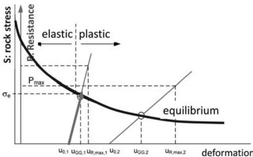
Figure 9. Ground-response-curve.
