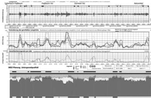
Figure 6. Example of the NATAS (new Austrian track analysing system) chart – overlay of track measuring signals and georadar information.
