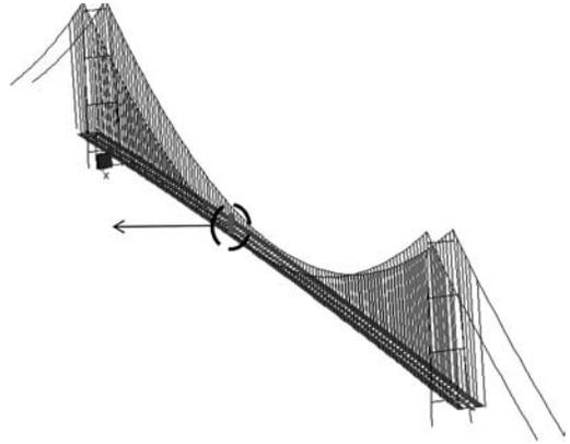
Figure 1. FE model of the bridge and positioning of the EH device.
