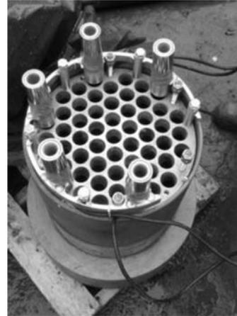
Figure 2. Sensor position on anchorage.
