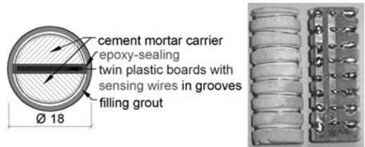
Figure 1. Filament-corrosion sensor with half-rounded PCC-mortar pieces for drill-hole installation, left: Sectional sketch of a double sensor, right: Photo with sensor's front and rear side.
