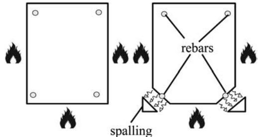
Figure 1. Cross-section with and without consideration of spalling effects.
