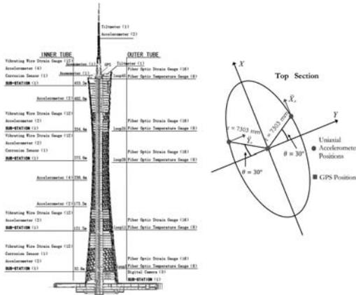
Figure 1. a) Actual tower instrumentation pattern taken from (<http://www.cse.polyu.edu.hk/benchmark/index.htm>), b) Location of the assumed measurement points for both GPS and accelerometer sensors.
