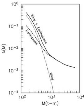
Figure 1. Exceedance rates of the bending moment acting in a wind turbine steel supporting structure, produced by wind, earthquake and both actions.
