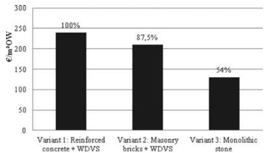
Figure 2. Life-cycle cost analysis of the investigated three variants of wall construction.
