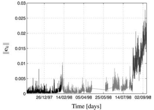
Figure 2. Z24 bridge, misfit of the nonlinear output-only model. Black: Training data. Light gray: Monitoring data in undamaged condition. Dark gray: Monitoring data in damaged condition.
