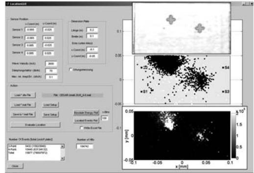
Figure 1. GUI of a Matlab code (overall), color coded AE energy distribution for a 20 J impacted panel loaded for 100 cycles (bottom right) and US C-scan for a 20 J impacted panels (top right).
