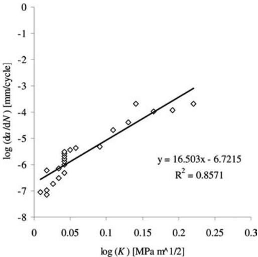
Figure 1. Relation between measured  $da/dN$  and  $K$  for specimen made from C30/37 concrete.
