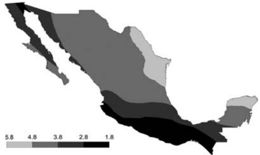
Figure 2. Map of reliability indexes considering seismic action on wind turbine studied for  $S_L = 10$ .
