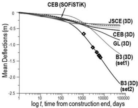
Figure 4. Deflection curves for the KB Bridge computed with finite elements using various creep and shrinkage models. The data shows a linear trend in logarithmic time.
