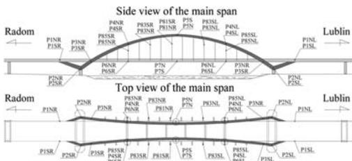
Figure 1. Localization of test points on the bridge.
