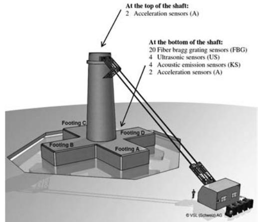
Figure 1. Sensors at the gravity base in Cuxhaven.
