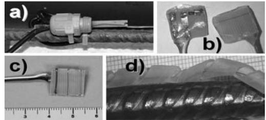
Figure 2. Further developments of the filament-sensor: a) and b): 1-wire sensors as elements of a 2D-sensor array, c) 3-wire sensor with varying wire diameter as a corrosion threshold value sensor, d) distributed, long gage sensor in a spiral hose.
