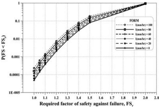
Figure 1. The relationship between required factor of safety and failure probability for different rainfall intensity ( $T = 36$  hr).
