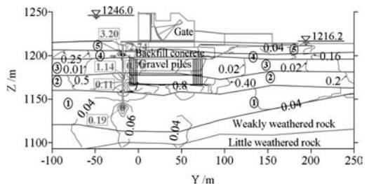
Figure 2. Hydraulic gradient contour at the section of the gate.
