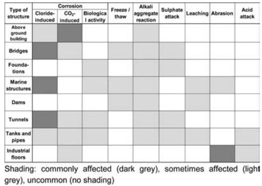
Figure 3. Predominat deterioration mechanisms for different concrete structures, Buenfeld et al. (2008).
