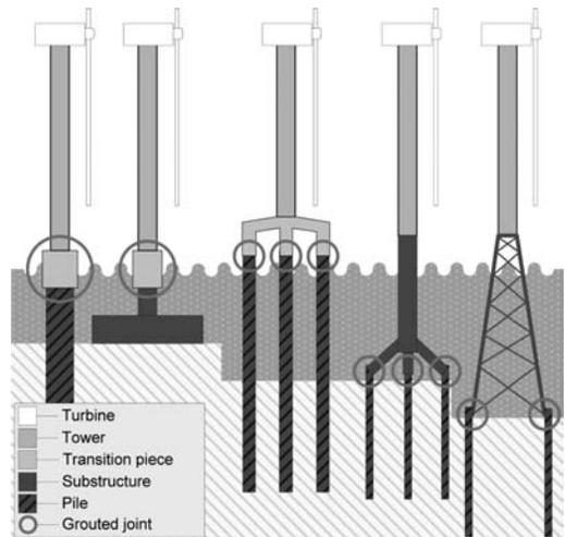
Figure 1. Supporting structures, from left to right: monopile, gravity based foundation, tripile, tripod, jacket.
