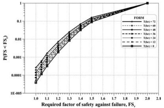
Figure 2. The relationship between required factor of safety and failure probability for different rainfall duration ( $I = 50$  mm/hr).
