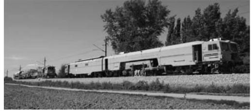
Figure 3. MDZ machinery at work (tamping machine, track stabiliser, ballast distribution system).
