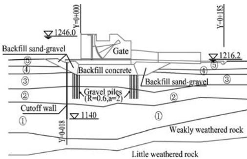
Figure 1. Typical cross section of the gate.
