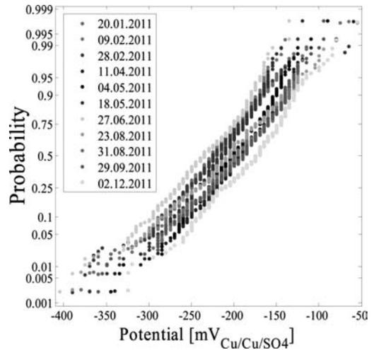
Figure 1. Probability plots of all measurements in 2011 with the same pre-wetting condition after Guideline B3.
