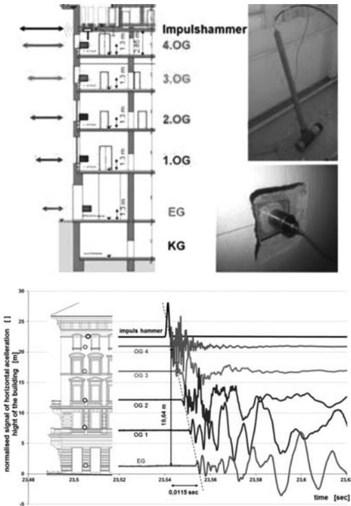
Figure 1. Experiment for wave dispersion in masonry wall.
