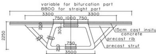
Figure 1. Box girder section used in the APM project in PNU.
