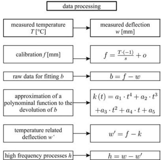
Figure 1. Separation process of measured data into individual portions.
