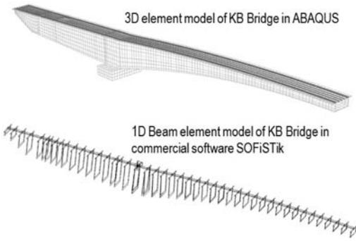
Figure 3. 3D Finite element models of the KB Bridge using ABAQUS and SOFiSTik.
