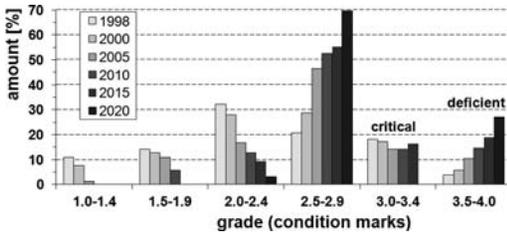
Figure 2. Expected condition development of German highway bridges without enhanced maintenance.
