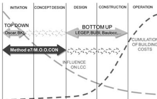
Figure 1. Missing link in models for calculating life-cycle costs during the design phase (Source: original illustration).
