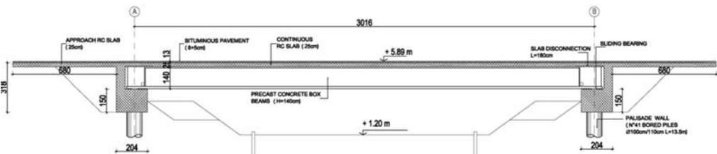
Figure 1. Joint-less Bridge on the River Musestre: Transverse section and plan.
