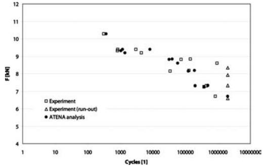
Figure 2. Comparison of measured and calculated results for C45/55 class concrete.
