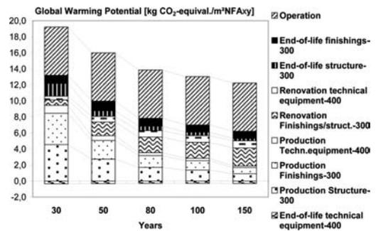
Figure 1. GWP. Phases: production, operation, replacement/renovation and end of life (for technical equipment, load bearing structure and finishes).
