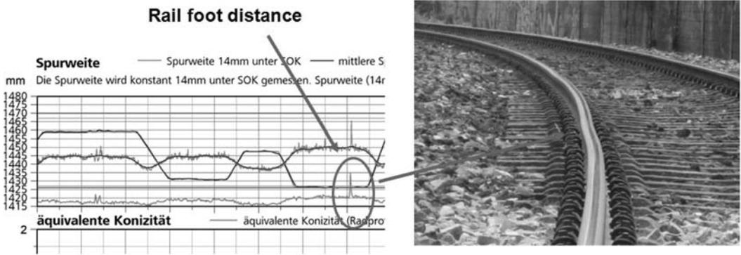
Figure 8. With the measuring signal rail foot distance the track masters can easily find sections with a poor condition of the fastening system.
