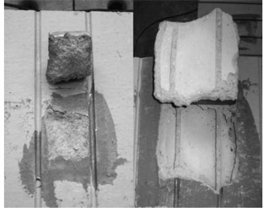
Figure 1. Stone break-out on tests with vertically perforated bricks.
