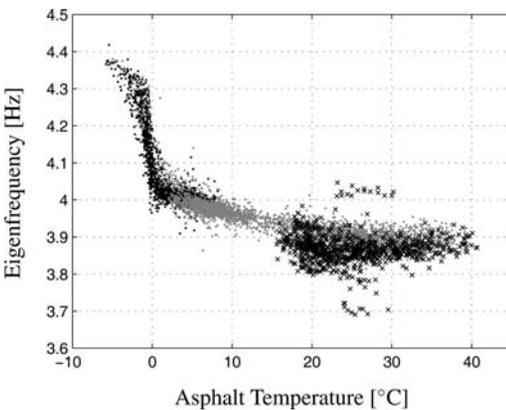
Figure 1. Z24 bridge, fundamental natural frequency as a static function of the temperature of the asphalt layer. Black dots: Training data. Grey dots: Monitoring data in undamaged condition. Black crosses: Monitoring data in damaged condition.
