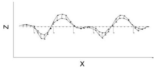
Figure 3. Identified mode shape of Mode 3 (4.16 Hz, 1.3%).
