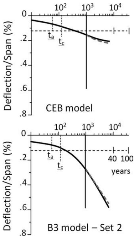
Figure 6. Deflection estimates applied to the predictions of the KB Bridge deflection obtained from 3D FEM studies. The dashed line is the estimate and the solid line is the computational solution.
