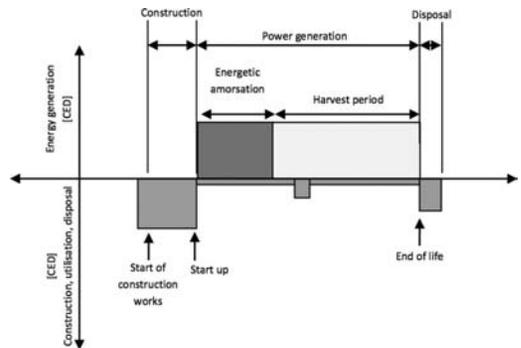
Figure 2. Illustration of determining the harvesting factor.
