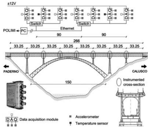
Figure 1. Elevation and cross-section of the San Michele bridge and schematic of the monitoring system (dimensions in m).
