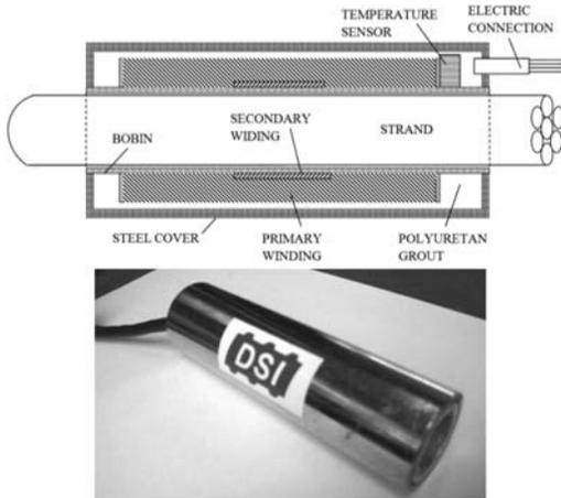
Figure 1. Design of the sensor.
