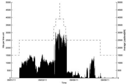
Figure 1. Htrate from an AE Sensor during a load scenario.
