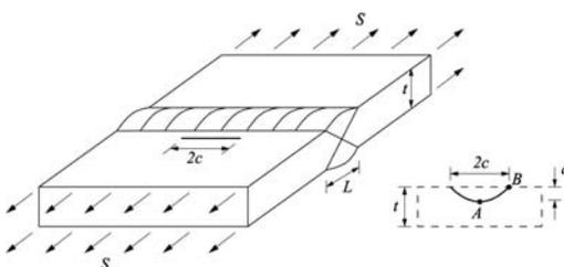
Figure 1. Butt welded plate containing a semi-elliptical surface crack in the weld toe region.
