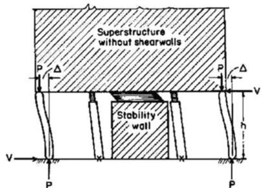
Figure 1. Sketch of a shock-absorbing first story during seismic motion. The columns and neoprene pads were expected to provide restoring forces (Drawing from Khan and Fintel, "Shock-Absorbing Soft Story," 1969).
