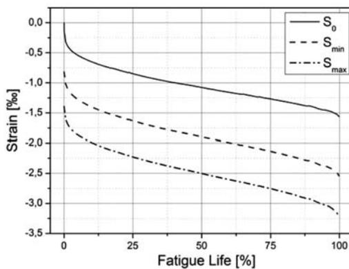
Figure 1. Longitudinal strains during life-cycle on different load levels (exemplary).
