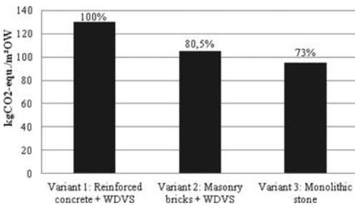
Figure 1. CO<sub>2</sub>-equivalents as an exemplary ecological effect of production, maintenance, and demolition of the investigated three variants of a wall construction.
