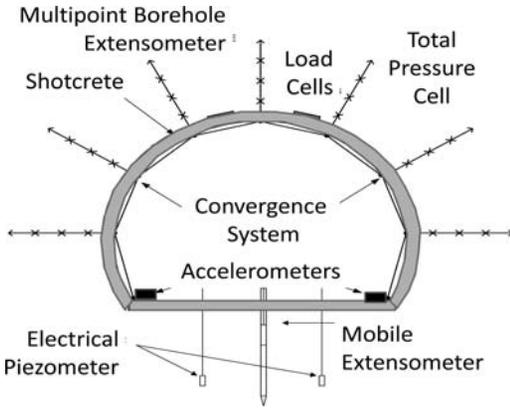
Figure 3. Typical instruments for tunnel monitoring.
