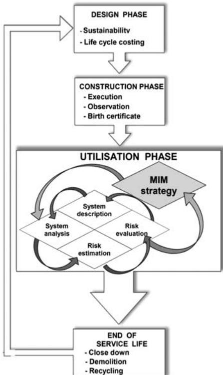
Figure 1. Life-cycle phases including Monitoring, Inspection and Maintenance (MIM) strategy (Horstmann et al., 2012).
