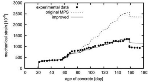
Figure 2. Evolution of mechanical strain of a sealed concrete sample subjected to several thermal cycles.
