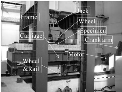
Figure 1. Wheel load traveling test equipment.
