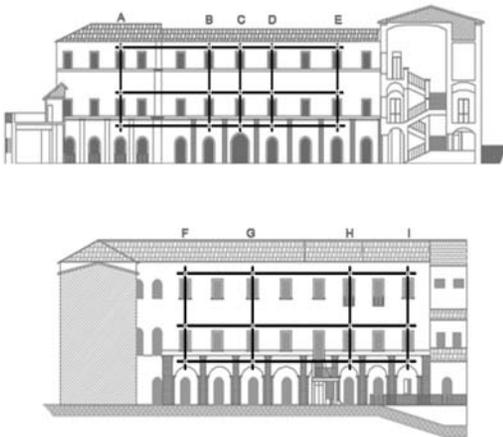
Figure 1. Grid of monitored points set on the building' SW (above) and NW internal fronts (below).
