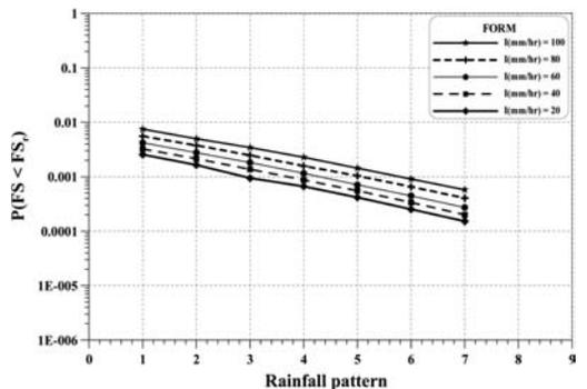
Figure 3. The relationship between rainfall pattern and failure probability for different rainfall intensity with  $FS_r = 1.2$ .
