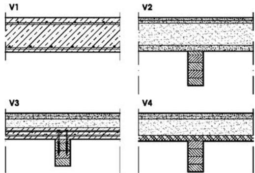
Figure 1. Schematic sections of floor structures alternatives.
