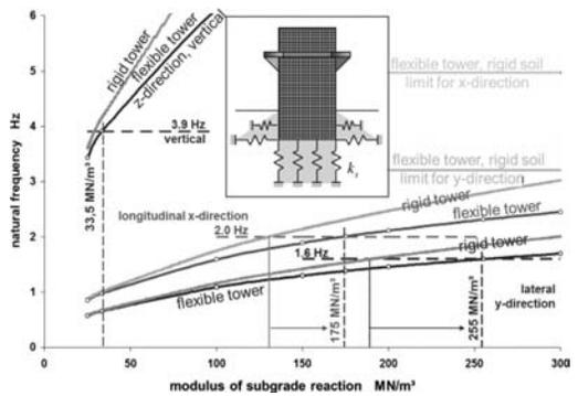
Figure 3. Coherency between modulus of subgrade reaction and Eigenfrequency for different modes of vibration for rigid body movement and elastic building characteristic, comparison of FE-computations with measured results.
