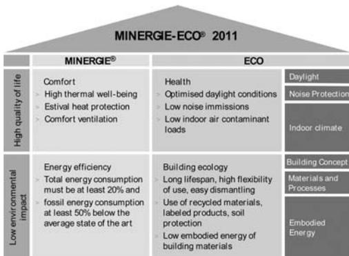
Figure 1. Newly structured criteria of MINERGIE-ECO<sup>®</sup> 2011.
