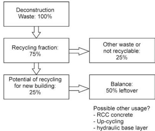
Figure 1. Material stream of deconstruction waste. About 75% of the total waste are recyclable. In the end, about 50% are leftover. The balance could be enhanced with the help of other products which make use of recycled crushed mineral waste.
