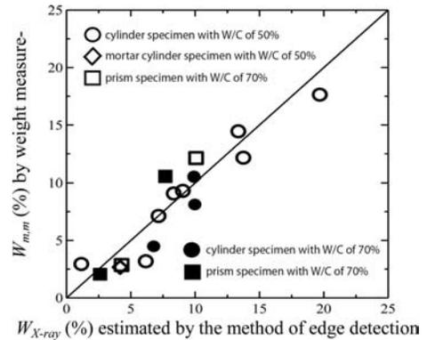
Figure 2. Comparison of steel weight loss by weight measurement ( $W_{mm}$ ) with that estimated by the digital image processing ( $W_{X-ray}$ ).
