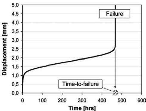
Figure 1. Creep-to-failure curve of an epoxy based bonded anchor system under a static load.
