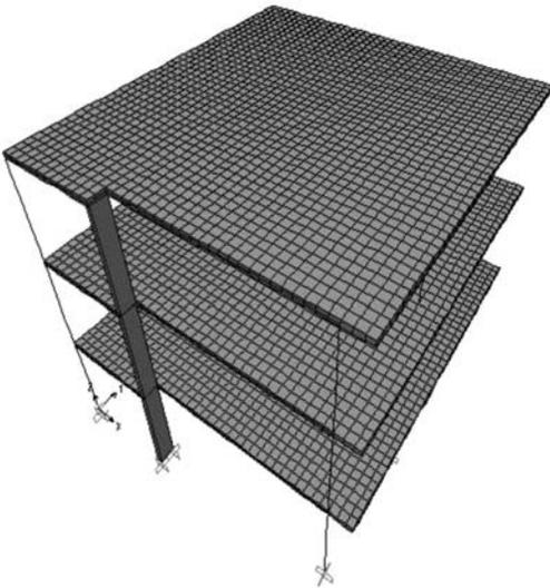
Figure 1. FE Analysis model of the SPEAR structure.
