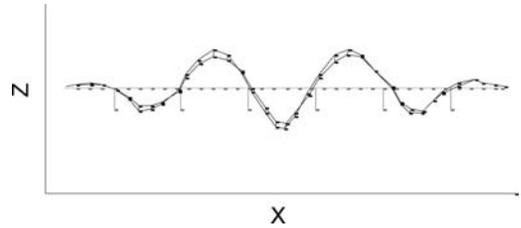
Figure 2. Identified mode shape of Mode 2 (3.76 Hz, 0.8%).
