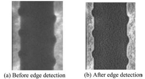
Figure 1. Detection of edge between rebar and concrete.
