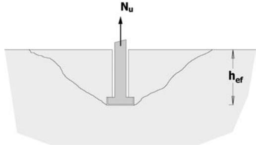
Figure 1. Single anchor failing with concrete cone breakout.
