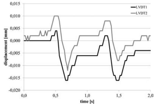
Figure 1. Displacements measured in the direction of the corresponding pairwise transducers caused by a crossing single railcar type 5047.
