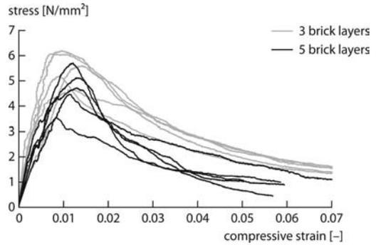
Figure 1. Stress-displacement relations from compression tests on column-type test specimens.
