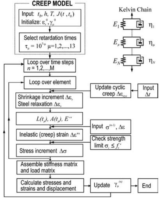
Figure 2. Kelvin chain model and flow chart of the algorithm of finite element creep analysis based on rate type creep model.
