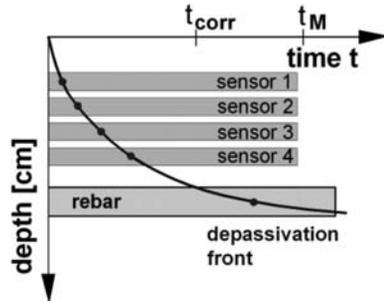
Figure 7. Operating principle of integrated corrosion sensors in different depths within the concrete cover of a rebar with  $t_{corr}$  = corrosion initiation (depassivation) time and  $t_M$  = maintenance (rehabilitation) time, if  $t_M < t_{service\ life}$ .
