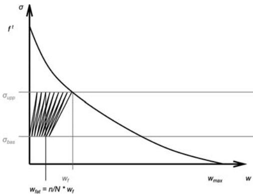
Figure 1. Softening law vs. crack opening displacement and fatigue damage.
