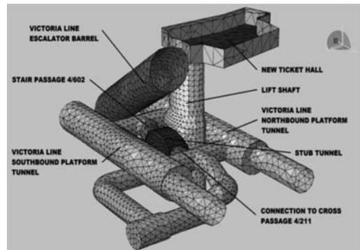
Figure 1. Model of the Green Park Station in London; new and existing structures.
