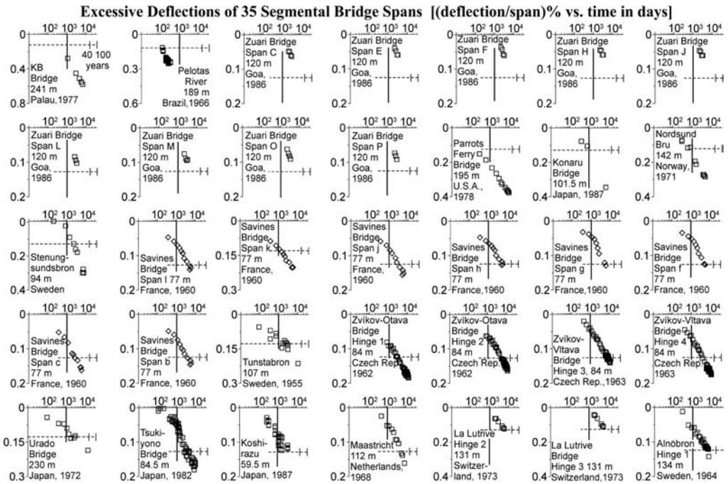
Figure 5. A collection of logarithmic time scale plots of the bridge deflection records. A linear trend is observed beyond the marked 1000 day line. The horizontal dotted line represents the excessive deflection limit.
