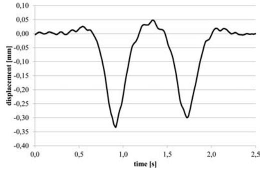
Figure 1. Vertical displacements caused by a crossing single railcar type 5047, determined by laservibrometer.
