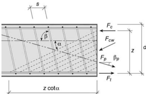
Figure 1. Stress field in girder web with variable inclination of compression fields, according to SIA 262 (2003).
