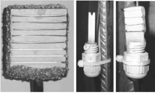
Figure 8. Innovative filament sensors for integrated corrosion monitoring of concrete structures – corrosion initiation sensor: a): deep dependent 5-wire sensor in the concrete cover, b): single steel wire sensor mounted at a rebar and c): multi-wire corrosion progress sensor at rebar with different wire diameters, cp. Holst & Budelmann (2012).
