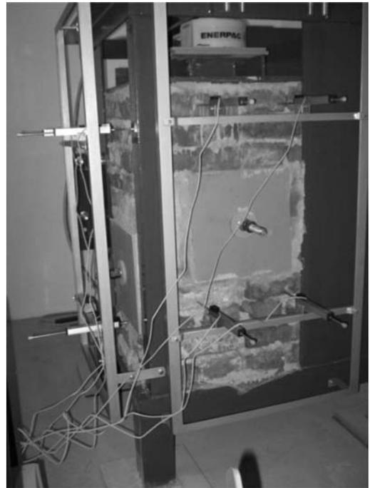
Figure 1. Testing equipment for pre-stressed masonry corner.
