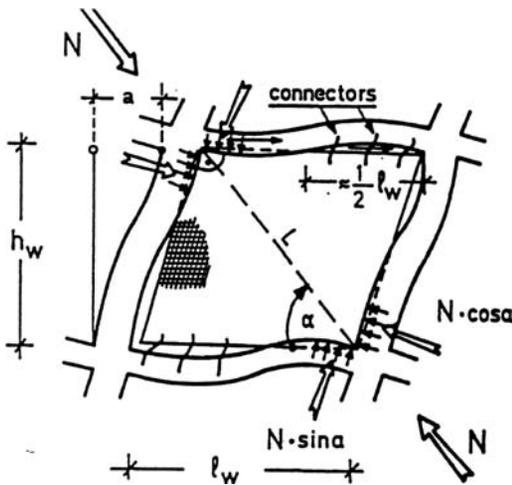
Figure 1. Deformed post installed shear wall at earthquake loading (Guidelines for Seismic Retrofit, 2001).
