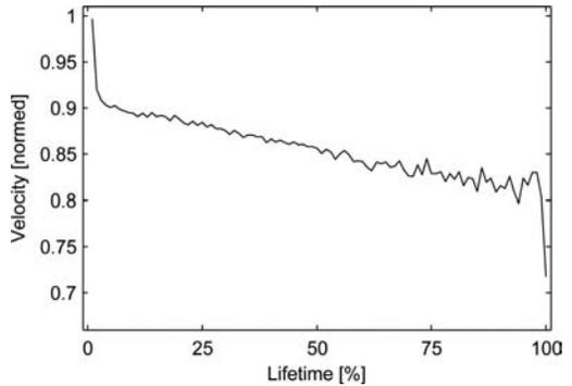
Figure 2. US-velocity over a small scale specimen's life time.
