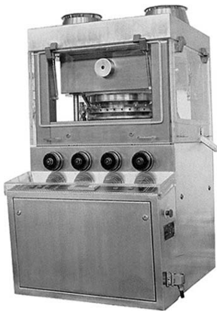
Figure 16.3 A typical high-speed automatic tablet-making machine. Note the full enclosure to help prevent contamination while allowing clear viewing of the press in operation. Courtesy of Tabletpress.net.
