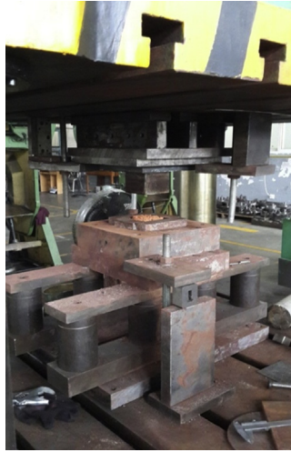
Figure 7.23 Press device for block formation of heavy metals and organic pollutants—contaminated construction and demolition waste.
