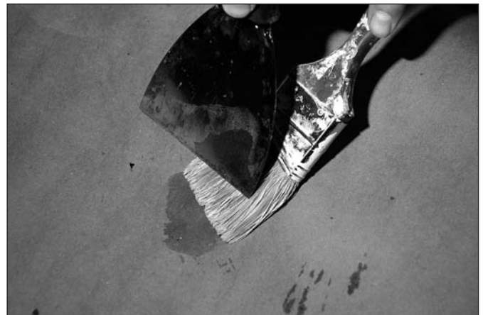
Figure 8-32: Person removing excess paint from brush
