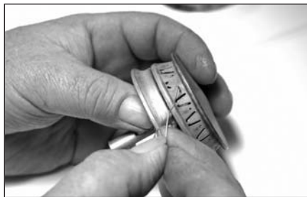
Figure 11-2: Cleaning pilot holes on gas burner
