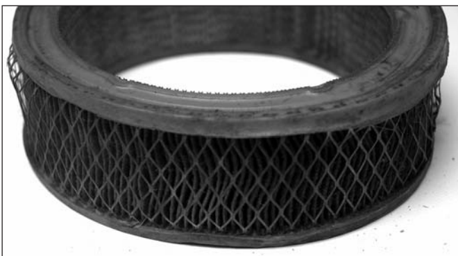
Figure 15-33: Dirty air filter
