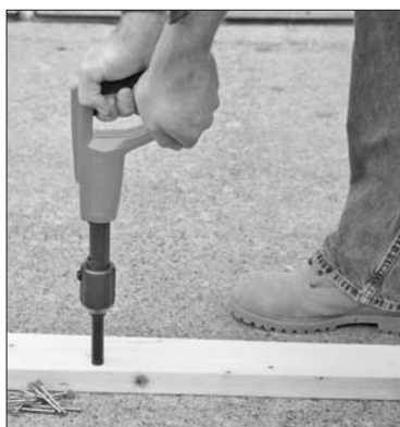
Figure 7-7: Power-actuated drivers are used for fastening into masonry or steel
