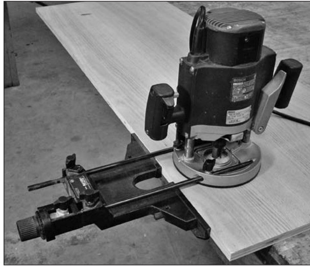
Figure 4-43: A guide attached to the base of the router rides along the edge of the stock and controls the sideways motion of the router
