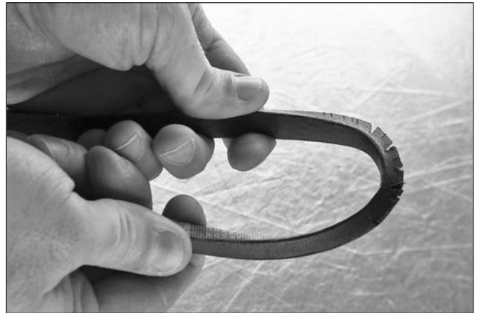
Figure 10-5B: This belt is cracked and needs to be replaced
