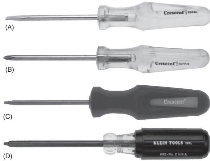
Figure 4-29: Screwdrivers: (A) slotted, (B) Phillips, (C) torx, and (D) square or Robertson
