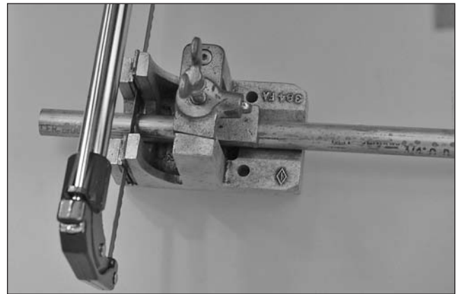
Figure 9-31: Copper tubing in fixture
