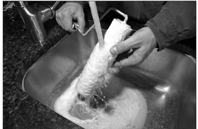
Figure 8-31: Rinse paint roller under tap
