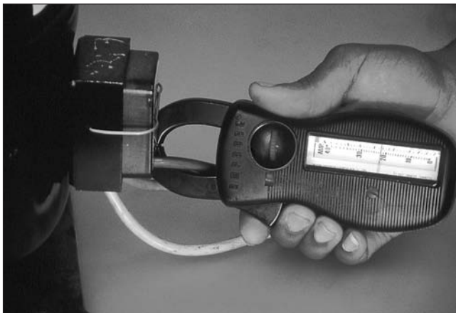
Figure 6-9: Measuring amperage by clamping the meter around the conductor. (Courtesy Bill Johnson)
