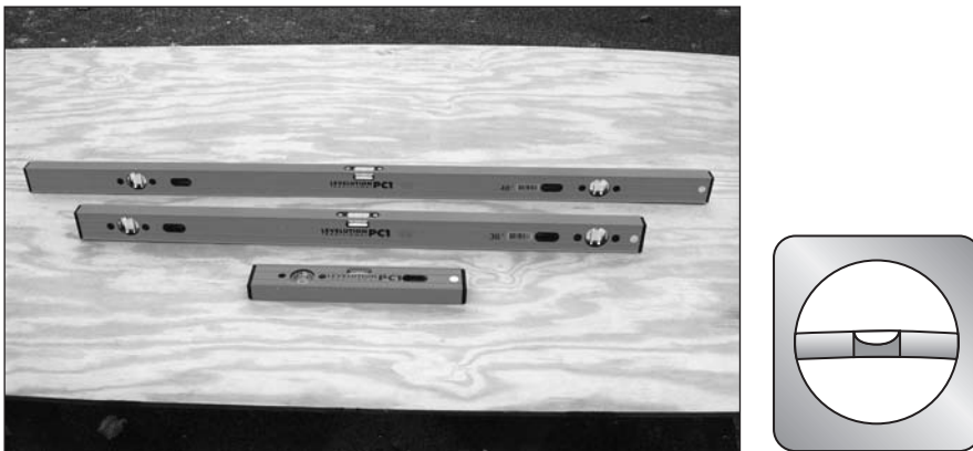
Figure 4-17: A spirit level has one or more transparent vials containing a liquid and a bubble
