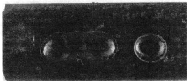
Figure 2.8 Pitting on external surface of tubing in sour service—annulus was open ( i.e. , no packer).
