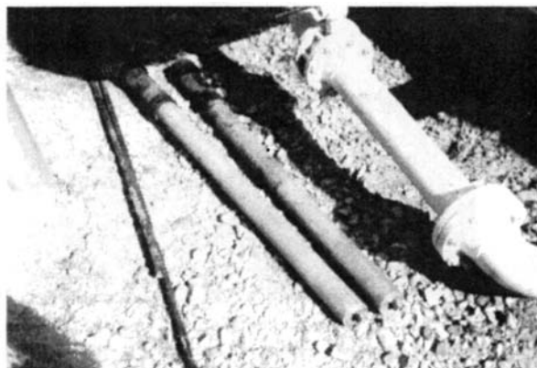
Figure 7.11 Galvanic anodes for insertion through a vessel wall. (Figure 7.12) The dark area at the top is the nonmetallic insulator, and the mounting head with the lead wires.
