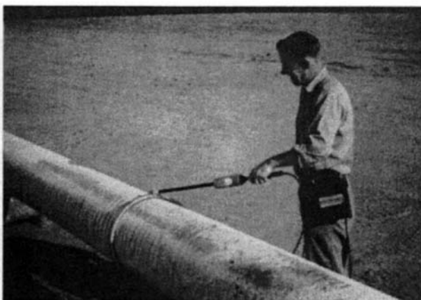
Figure 6.30 Holiday detection—High voltage ring type holiday detector inspecting a pipeline coating. (Photograph courtesy of KTA-Tator, Inc., Pittsburgh, PA. 38 )
