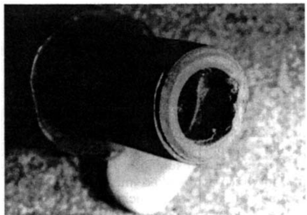
Figure 3.25: Bimetallic Corrosion (Galvanic Attack) —This steel nipple was screwed into a brass water meter at a waterflood injection well. The failure occurred after about 10 months of service.
