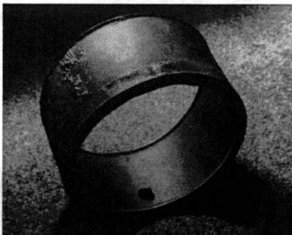
Figure 3.5 Pitting Corrosion —Isolated pit from gas well gathering line.
