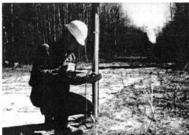
Figure 7.2 A technician taking a reading at a CP test station in a pipeline right-of-way. The copper-copper sulfate reference electrode, visible below his left knee, is placed in the soil for the reading. (Photograph courtesy Bass Engineering Co., Longview, TX. 2 )
