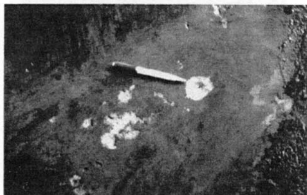
Figure 3.19 Underdeposit Corrosion— Pitted type 304 stainless steel tray clip from deaeration tower handling silty seawater. Solids deposited in the trays created differential aeration cells in the oxygen rich water. (Corrosion mechanism similar to that illustrated in Figure 3.12.)
