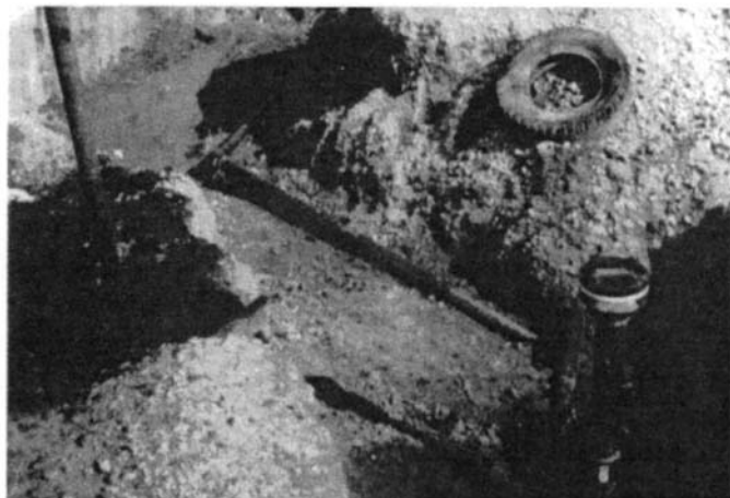
Figure 5.4 Polyvinyl chloride (PVC) plastic flowline on a sucker rod pumping well.
