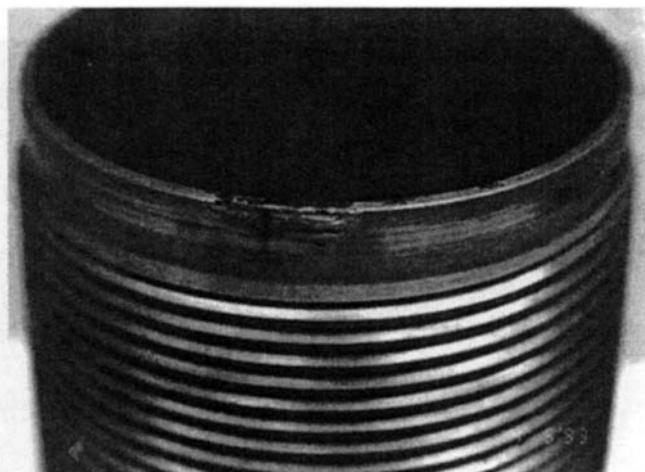
Figure 3.13 Concentration Cell Corrosion—Example of crevice attack in pipe joint. 2
