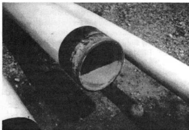
Figure 6.29 Pipeline coating—Extruded polyethylene coating.
