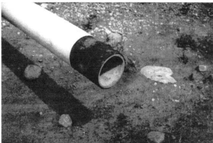
Figure 6.25 Cement lined pipe for a water injection system. Note extruded external coating.
