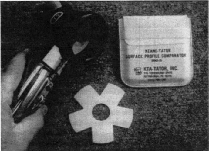
Figure 6.14 Surface profile with replica tape. (Photograph courtesy of KTA-Tator, Inc., Pittsburgh, PA. 14 )
