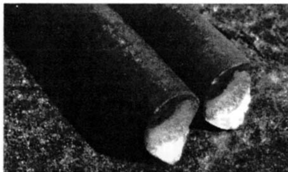
Figure 3.46 Corrosion Fatigue—Failed sucker rod. The most common cause of sucker rod breaks. Note the three areas of the failure: the smooth area where the cyclic action "peened" the surface, the grainy looking area where the crack opening was too fast for the "peening" to take place, and the final tip where the cross sectional area had been reduced to the point where the rod would handle the load and thus failed in a typical tensile failure fashion.
