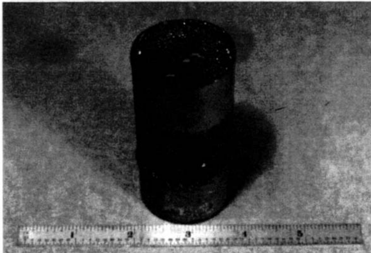
Figure 3.11 Pitting Corrosion—Severely pitted copper hot water line from crew quarters.
