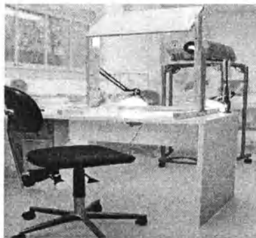
Figure 1. One of our Gesture Modelling configurations: camera and gesture space beneath the desk, with lights, projector and mirror displaying the model image on the desk top.
