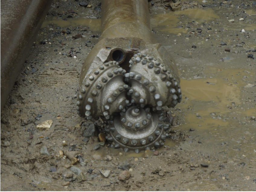
Plate 2.3 Roller bit that cut through soil. A hole is provided to send water to keep the bit cool.
