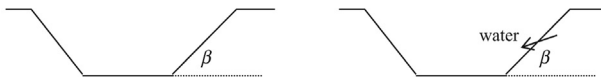
Figure 28.1 Unbraced excavations. (a) Rounded coarse sand, (b) sand with water emerging from slope.
