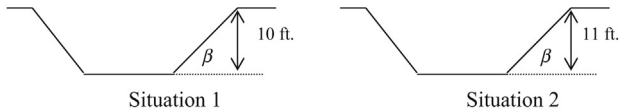
Figure 28.2 Embankments. Situation 1: silty clay (PI = 12) and use table 20.2 to obtain \beta = 39^{\circ} . Situation 2: clayey silt (PI = 8) and use table 20.2 to obtain \beta = 32^{\circ} .
