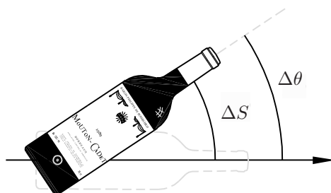
FIGURE 35.1 Angular Motion of a Rigid Extended Body and the Rectilinear Motion of a Reference Point
