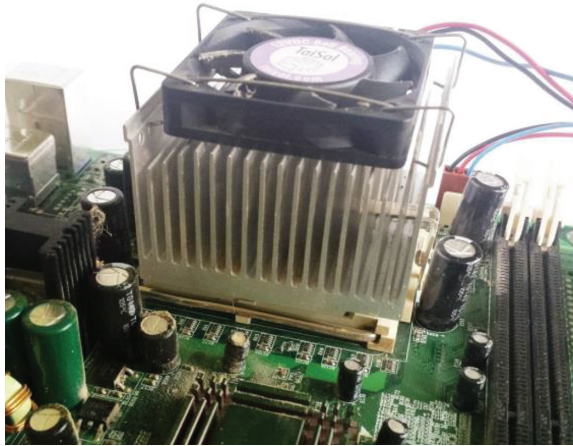
FIGURE 6.5 Aluminum heat sink with a fan in a computer circuit board.
