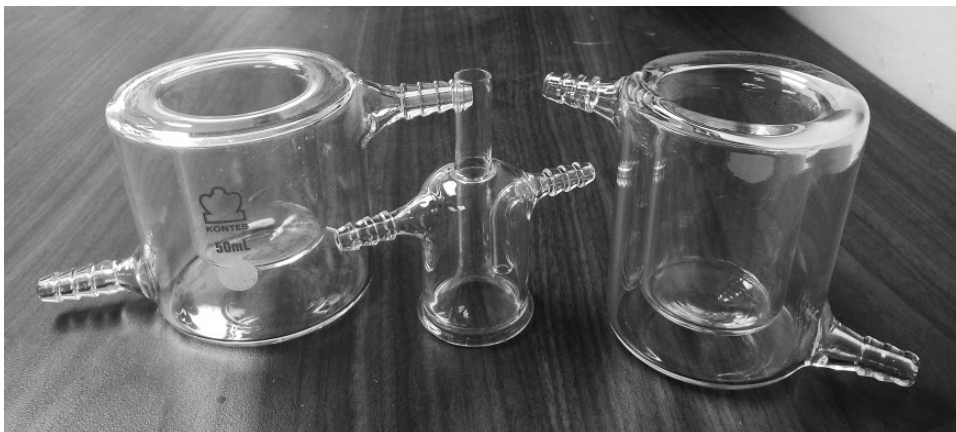
Figure 21.2 Commercially-available glass feeders used for feeding bed bugs in vitro .
