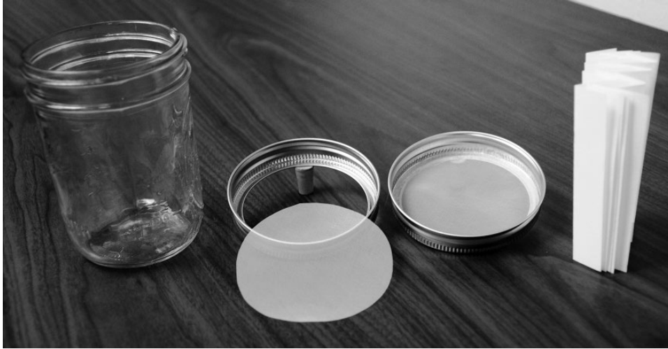
Figure 21.1 Mason jar and components used to house bed bugs. Unassembled and assembled cap with mesh screening, and folded, filter paper harborage.
