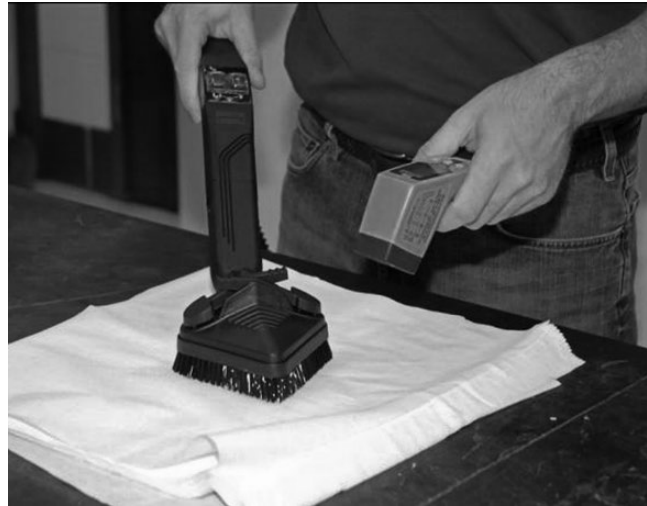
Figure 28.2 Use of an infrared thermometer to verify surface temperatures immediately after steam application. (S.A. Kells, University of Minnesota).
