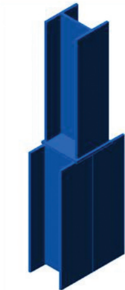
Figure 18.8 Possible perimeter column splice to achieve flush internal space, see circle in Figure 18.9
