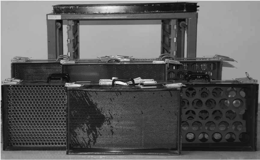
3.2 Equipment for determination of the particle size distribution of woodchips with a nominal top size above 3.15 mm.
