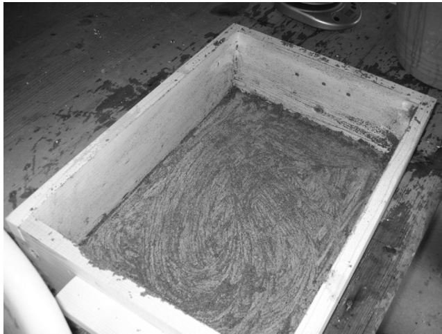
Figure 16.1 Typical wooden mold used to make an adobe block. The mold is first wet with water and scattered inside with sand so as to reduce water absorption by wood and facilitate the removal of the earth block.
