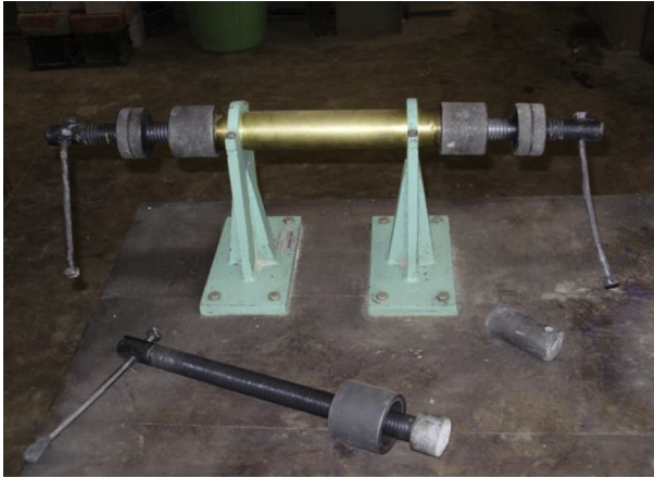
Figure 15.2 Static compaction device.
