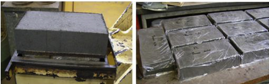
Figure 18.8 Clay–PFA “Eco-brick” made sustainable by using the already proven sustainable lime–GGBS blended binder.
