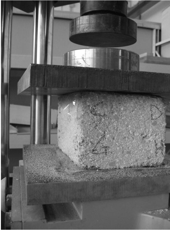
Figure 16.5 A typical compressive test on an adobe block specimen.
