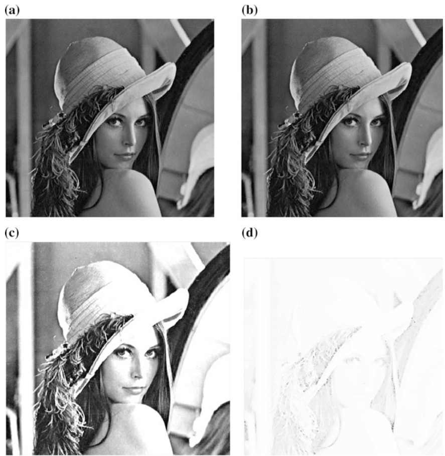
Fig. 4 a Input image I, b input image II, c output image obtained upon exact addition, d resultant image obtained after approximate addition
