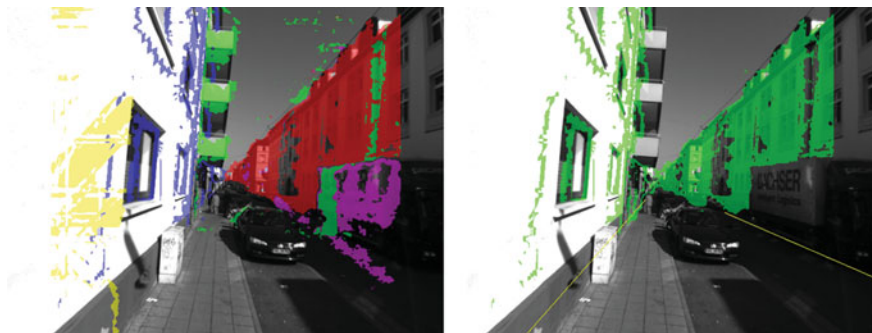
Fig. 16.3 RANSAC based planar segmentation. The two most parallel planes ( right ) are selected from five hypotheses ( left )
