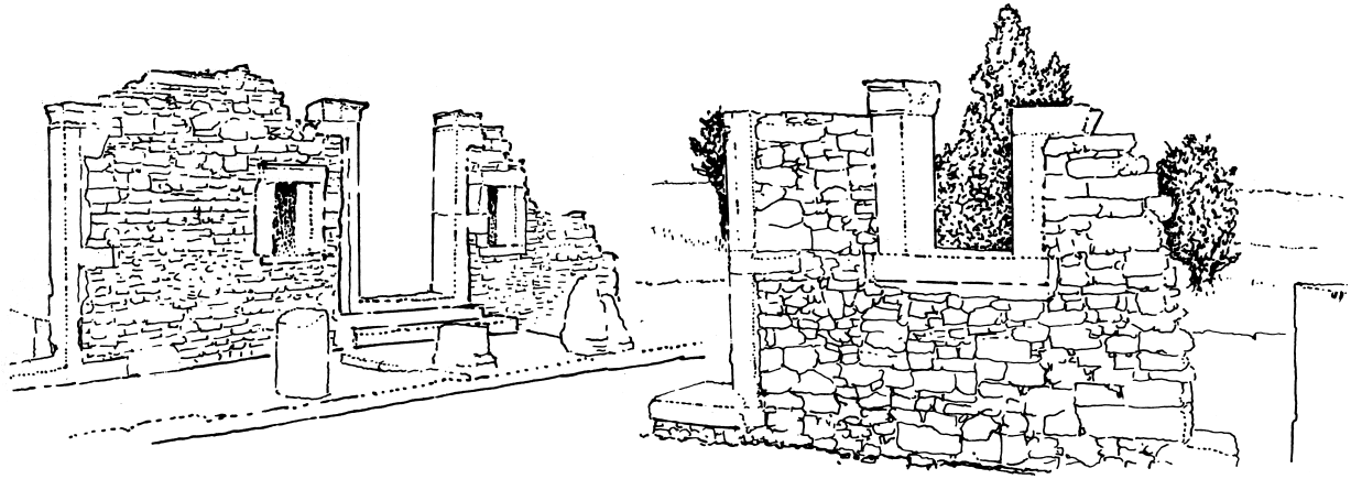
209. Kourion. Sanctuary of Apollo Hylates. Mixed Ashlar and Rubble Masonry. Cyprus. 1st Century AD. As opposed to Greek practice which was loathe to contaminate the perfection of ashlar by inferior association, Roman construction often employed ashlar elements to stiffen rubble walls in various fashions. One system (as shown here) was to stiffen rubble walls by ashlar coigning and framing to doors, windows. This very functional device recurred in numbers of contexts across the ages. After ABC II, fig 270.
