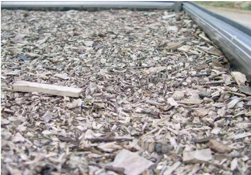
Fig. 3.10 Wood chips media (Source Hartmann Filter GmbH & Co.KG.)
