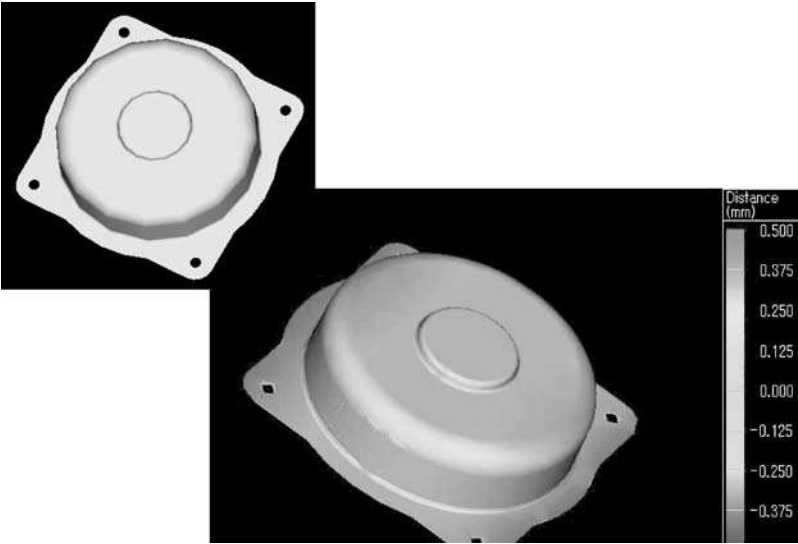
Figure 4.21 Example of CAT data converted to XVL
