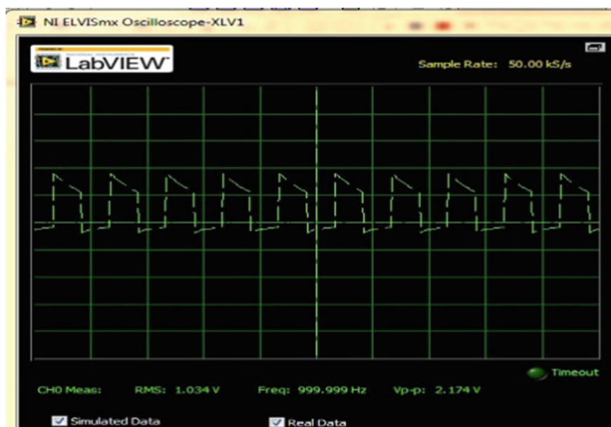
Fig. 6 Response of clamper circuit
