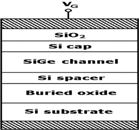
Fig. 2 SiGe MOS structure used in simulation
