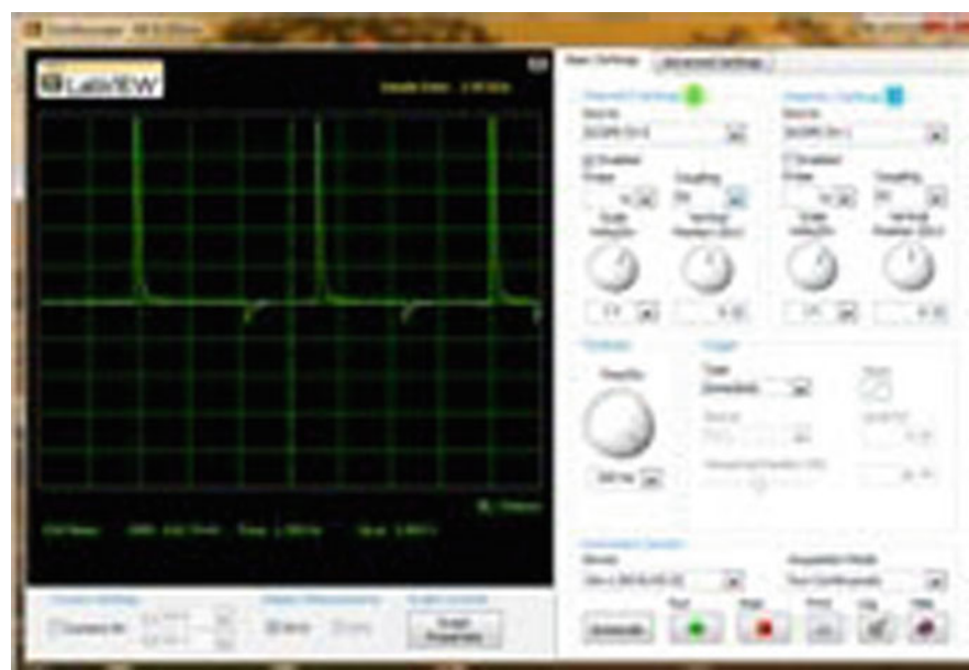
Fig. 10 Output from the negative clamper Patient 3 under physical exertion
