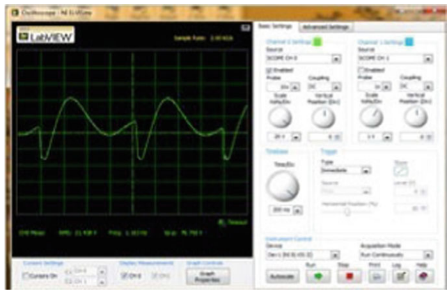
Fig. 8 Above image depicts the ECG waveform and its frequency of Patient 2 as derived from our system design setup
