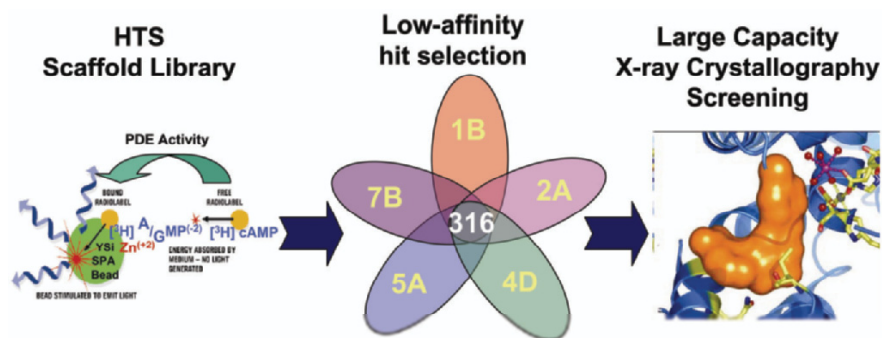
Figure 6-4. Low-affinity screening against multiple members of a protein family. Compounds in the scaffold library are screened against multiple members of a protein family using a biochemical assay in HTS format. For example in PDEs, a scintillation proximity assay is used to screen against PDE1B, PDE2A, PDE4D, PDE5A and PDE7A with compounds at 200 \mu\text{M} concentration. Only those 316 compounds that showed above 30% inhibition against at least three out of the five PDEs in the screening panel are selected for further screening by co-crystallography.
