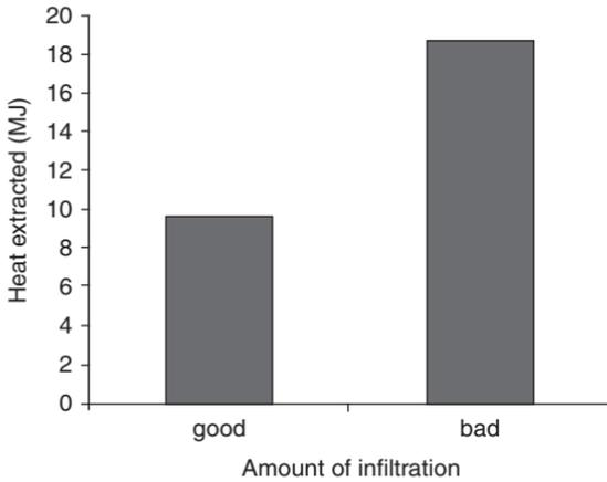
**Fig. 9.5** Heat extracted by the refrigeration plant during the standard journey for a well, and a poorly sealed van (source: Gigiel, 1998).
