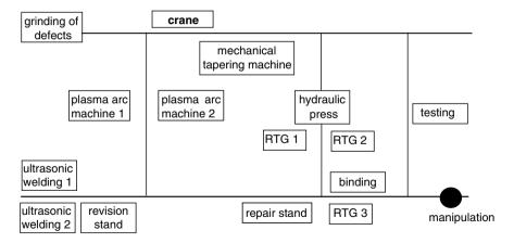
FIGURE 8.4 The arrangement of pipe mill hallis.
