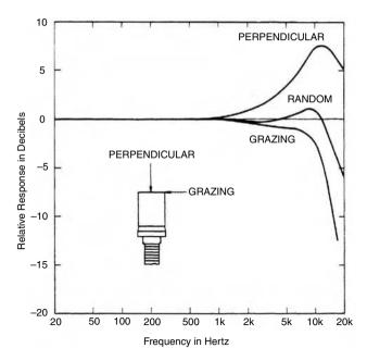
**FIGURE 31.5** Frequency response of an hypothetical microphone for three angles of incidence. (Adapted from Peterson, A.P.G. (1979). Noise measurements: Instruments. In Harris, C. M. (Ed.), *Handbook of Noise Control* [pp. 5-1–5-19]. New York: McGraw-Hill. With permission.)
