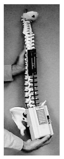
**FIGURE 49.1** The industrial lumbar motion monitor (iLMM), compared with an anatomical model of the spine.
