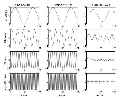
**FIGURE 12.4** LTI response to sinusoidal input signal with four frequencies  $\omega_0$  (left column), for two values of the variable  $\tau$ :  $\tau=0.1$  sec (middle column) and  $\tau=10$  sec (right column).
