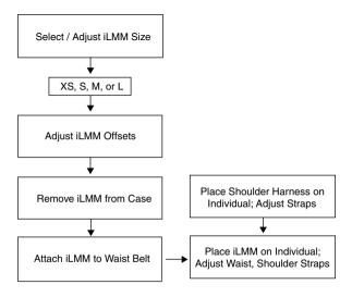
FIGURE 49.7 Flow chart of the iLMM setup procedure.
