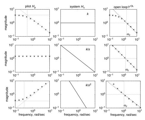
**FIGURE 12.11** Identification of pilot control behavior when controlling the three basic systems k, k/s, and  $k/s^2$ . The crosses indicate the frequencies of the sinusoids in the forcing function  $R(j\omega)$ . The dashed lines in the right column indicate integrator-like dynamics.
