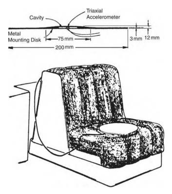
**FIGURE 33.4** Whole-body vibration vehicle measurements using an instrumentated seat disc. (Adapted from Wasserman, D. 1987. *Human Aspects of Occupational Vibration*, Elsevier Publishers, Amsterdam, The Netherlands. With permission.)
