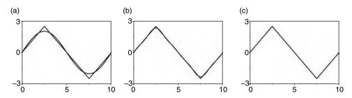
**FIGURE 12.8** Triangular function approximated by sums of sine functions, base frequency 0.1 Hz, following sine components at 0.3, 0.5, 0.7 Hz, etc. (a) one sine function; (b) three sine functions; (c) ten sine functions.
