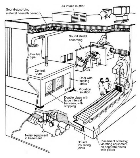
**FIGURE 31.9** Examples of noise control implementation in an industrial plant. (Adapted from OSHA (1980) *Noise Control, A Guide for Workers and Employers.* Occupational Safety and Health Administration Report No. 3048. Washington, DC: U.S. Department of Labor. With permission.)
