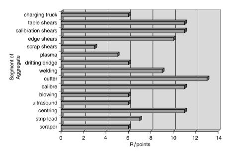
FIGURE 8.5 Technical risk analysis for all components of machine for ultrasonic welding 1.
