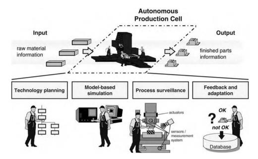
FIGURE 5.17 Autonomous production cell as work system.
