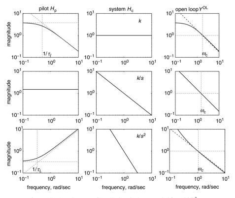
**FIGURE 12.12** Pilot equalization when controlling the three basic systems k, k/s, and  $k/s^2$ .
