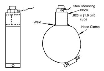
**FIGURE 33.5** Hand-arm vibration tool measurements using an instrumentated automotive hose clamp. (Adapted from Wasserman, D. 1987. *Human Aspects of Occupational Vibration*, Elsevier Publishers, Amsterdam, The Netherlands. With permission.)
