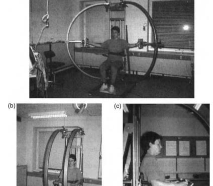
**FIGURE 14.3** Experimental chair, where arm posture can be adjusted in any position of abduction (a) and flexion (b). The hands are grasping handles connected to three-dimensional force transducers (c). Professor Bjørn Quistorff, University of Copenhagen, is acknowledged for the design.
