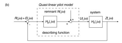
**FIGURE 12.10** The quasi-linear pilot model in the elementary single-axis compensatory tracking task. In this figure,  $H_c$  depicts the dynamics of the system to be controlled, and R, E, U, and Y the reference signal, the displayed error signal, the pilot control signal, and the system output signal, respectively. The quasi-linear pilot model consists of a describing function  $H_p$  and a remnant N, (a) single-axis compensatory tracking task; (b) quasi-linear pilot model.
