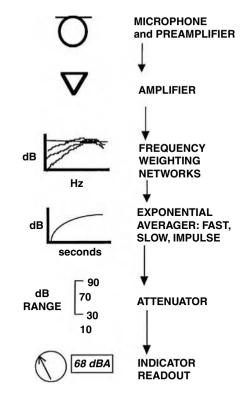
**FIGURE 31.4** Block diagram of the basic functional components of a sound level meter.
