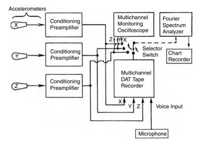
FIGURE 33.3 Basic triaxial vibration acceleration measuring system.
