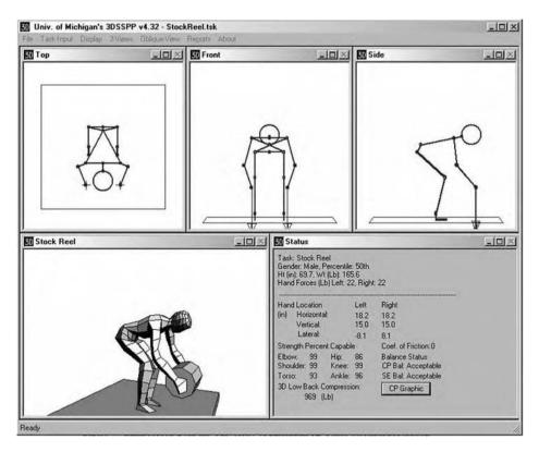
**FIGURE 48.7** Main screen from the University of Michigan 3D Static Strength Prediction Program for personal computers shown lifting a 44-lb stock reel. (With permission, Regents of the University of Michigan.)
