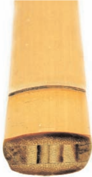
Figure 2.2. The layers of the Japanese yumi—bamboo inner core, mulberry wood on the borders of inner core, and bamboo back and belly.
