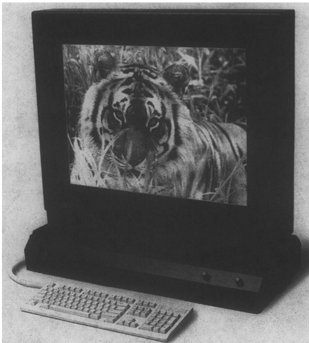
FIGURE 93.4 The 40 in. diagonal ac-driven plasma display from Photonics Imaging. (From Friedman, P.S., Inf. Display , 11(10), 22, 1995. With permission.)
