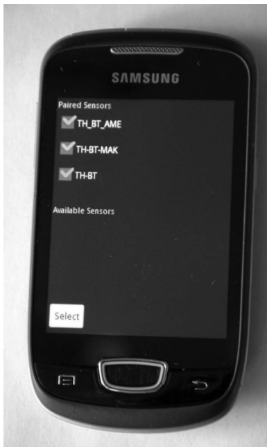
FIGURE 73.4 “Select Sensor” part of the new android application (aBluSen) for selecting several available sensors.
