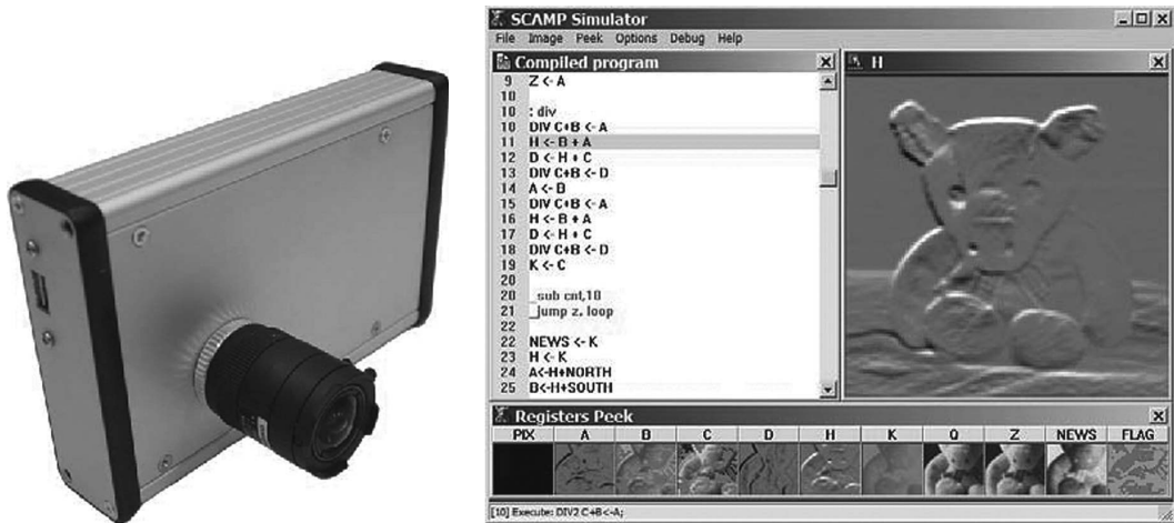
FIGURE 4.23 SCAMP-3 programmable vision chip.
