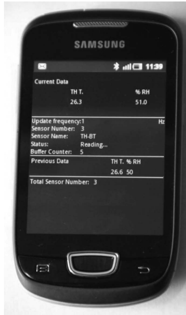
FIGURE 73.5 “Display” part of the new aBluSen application for the android’s mobile phone that shows the current and last data of the temperature and humidity values of the two sensors at the same time.
