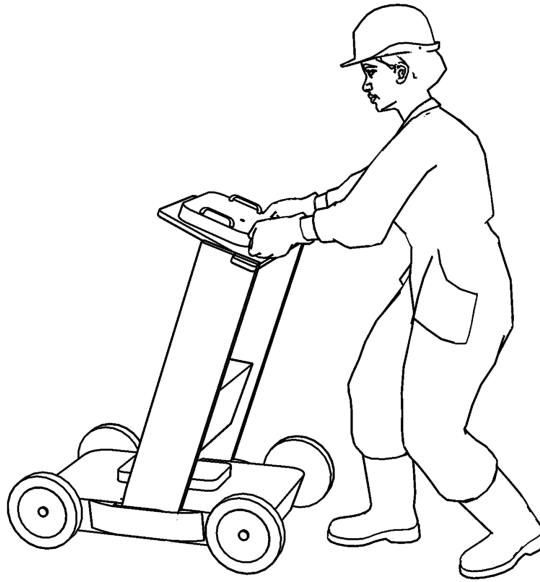
FIGURE 70.2 Typical cart-mounted utility-detection GPR.
