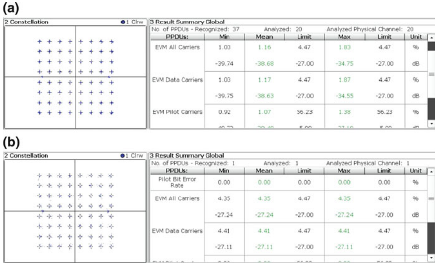
Fig. 6.18 EVM of an OFDM-64 QAM-modulated signal versus PA output BO from the P1dB compression point at 5500 GHz: (a) RMS data EVM of -38.63 dB at a 12-dB back-off from P1dB of 28 dBm and (b) RMS Data EVM of -27.11 dB at a 4-dB back-off from P1dB
