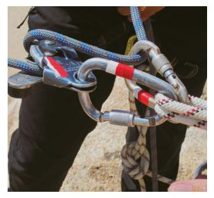
A Grigri rigged for lowering with the brake strand redirected through a carabiner clipped to the master point.
