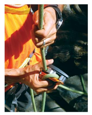
*The proper way to give slack quickly with a Petzl Grigri.*
