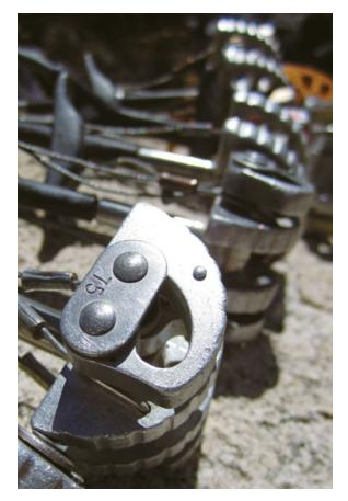
Spring-loaded camming devices have become an integral part of every climber's rack.
