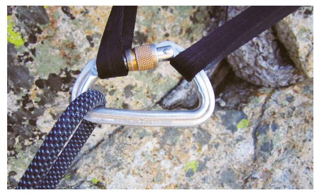
Very bad. Never load a carabiner on the minor axis or with a force outward on the gate.
