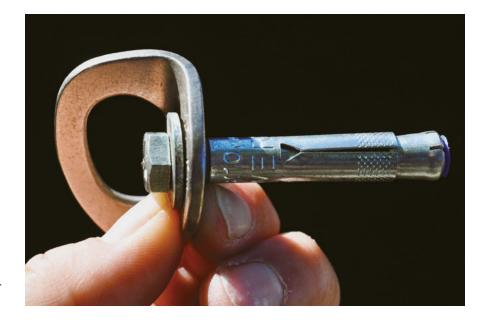
The <sup>3</sup>/<sub>8</sub>-inch diameter Powers Power Bolt expansion bolt with a stainless steel hanger has become the minimum standard for climbing anchor bolts.
