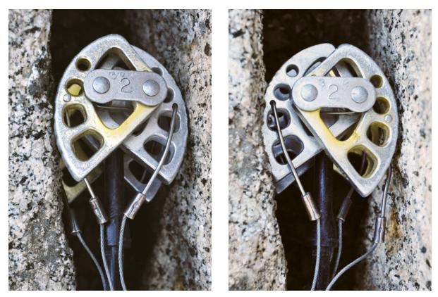
The same crack with two different placements. In the left-hand photo, the left outside cam has poor contact and is too close to the edge of the crack. By flipping the cam around (right photo), the gold cam now has flush surface contact with the rock. Since the inside and outside sets of cams are offset, flipping the cam one way or the other can often afford a better placement, particularly in shallow cracks in corners.
