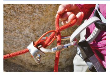
First pass a bight of rope through the carabiner and form a loop. If the device is under tension, pinching the rope against the device with the opposite hand will help lock it off.
