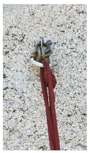
The cordelette is clipped directly to the bolt hangers with locking carabiners, bypassing the cheap hardware store lap links (which are only rated at around 1,000 lbs.).
