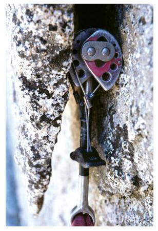
Bad. Any force applied to this Black Diamond Camalot will be converted to an outward force that can pry out and potentially break the flake of rock it's placed behind.
