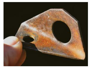
The recalled Leeper hanger can easily be identified by its unique shape and rusty condition.
