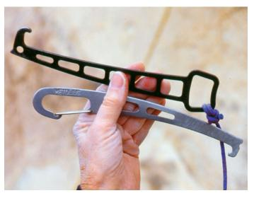
A nut tool is indispensable for removing chocks. Here are two models: Black Diamond (top) and Metolius (bottom).
