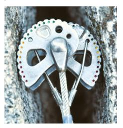
Borderline marginal. While this Metolius Power Cam is in a pocket that lends some stability to the placement, the range of retraction is between the yellow and red "range finder" dots; the red dots signify a marginal placement. The next larger unit would fit nicely.
