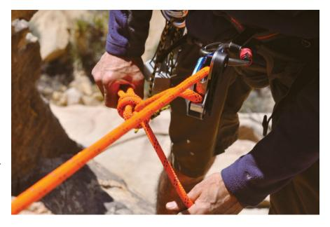
When using a Grigri on an instructor tether, tie an overhand knot backup whenever you take your brake hand off the rope. Always tie a stopper knot in the end of a rope tether to close the system.
