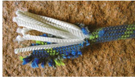
Deconstructed kernmantle rope showing the braided white interior core under the more tightly woven sheath.
