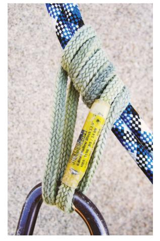
The Sterling Hollow Block, shown here wrapped in an autoblock configuration, is a 100 percent Technora sling designed specifically for use with friction hitches.
