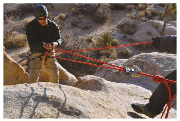
A 3:1 assisted raise. With the climber also pulling, there is a tremendous mechanical advantage, making it far easier to raise someone than with a 3:1 raise.
