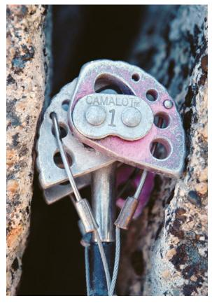
Bad. The two outside cams are not in the acceptable range for a Camalot (too wide), and they don't have flush contact with the walls of the crack.
