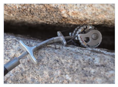
Camming units with flexible shafts are the best option for horizontal placement. Metolious recommends that in a horizontal crack, the outside cams should be placed on the bottom of the crack for maximum stability.
