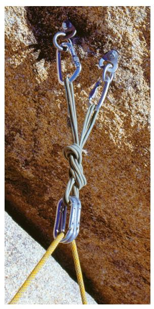
Simple two-bolt anchor rigged with a Tech cord (5,000 pounds tensile strength) cordelette. The cordelette is doubled to start with, producing four strands at the master point loop, and the climbing rope is clipped into three oval carabiners opposed and reversed.
