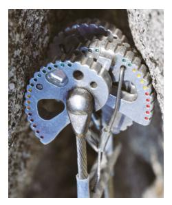
Bad. The crack is way too flared for this Metolius Power Cam, and the cam on the right side has very poor surface contact with the rock.
