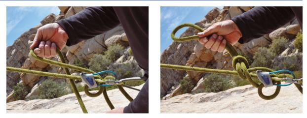
Then tie the mule knot above your device on the load strand of rope going to the climber.
