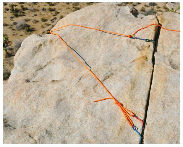
This finished rig illustrates the simplicity of the Joshua Tree System, with the lower leg connected to two anchors using a double loop figure eight. The upper leg was connected last, using a clove hitch to a locking carabiner for equalization, attached to two pieces and a doubled sling. Note the edge protector guarding both legs of the extension rope from abrasion.
