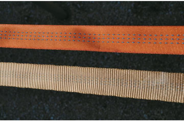
Top: Bluewater 1-inch climb-spec nylon webbing, rated at 18 kN tensile strength (4,047 lbs.). Bottom: REI 1-inch mil-spec nylon webbing, rated at 17.8 kN tensile strength (4,002 lbs.).
