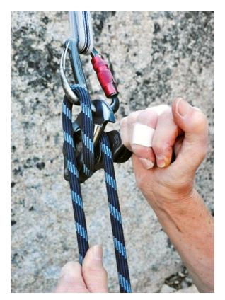
A Grigri in lowering mode with the brake strand redirected using the Petzl Freino carabiner, which is specifically designed for this application.
