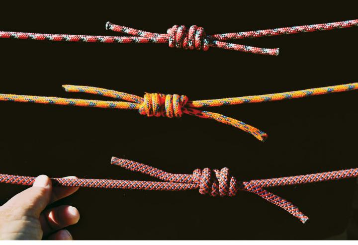
Cord Comparison. Top to bottom: Bluewater 5mm Titan Cord tied with triple fisherman's knot (Dyneema core/nylon sheath, tensile strength 13.7 kN or 3,080 lbs.); Sterling 6mm Powercord tied with triple fisherman's knot (Technora core/nylon sheath, tensile strength 19 kN or 4,271 lbs.); Sterling 7mm Nylon Cordelette tied with double fisherman's knot (nylon core/nylon sheath, tensile strength 12.4 kN or 2,788 lbs.).
