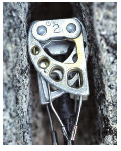
Borderline too tight. This Camalot is around 90 percent retracted. Any tighter and it may be very difficult to remove. There is also some loss of holding power in the last 10 percent (90 to 100 percent retracted) on a Camalot.
