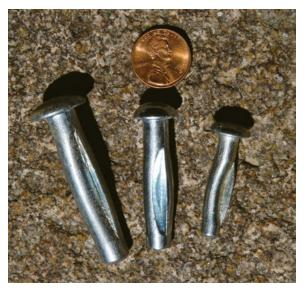
Buttonhead Rawl Drive contraction bolts (left to right): <sup>3</sup>/<sub>8</sub>-, <sup>5</sup>/<sub>16</sub>-, and <sup>1</sup>/<sub>4</sub>-inch sizes.
