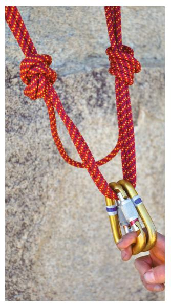
Detail of quad rig with two locking carabiners opposed and reversed.
