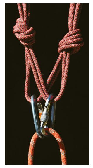
Detail of an equalette toproping rig tied with a doubled cordelette for a two-bolt anchor.
