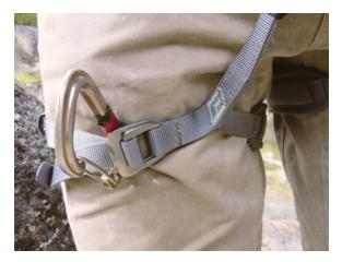
Note where the carabiner sits on the harness. Rigging an autoblock backup from this position has the potential to unbuckle the leg loop.
