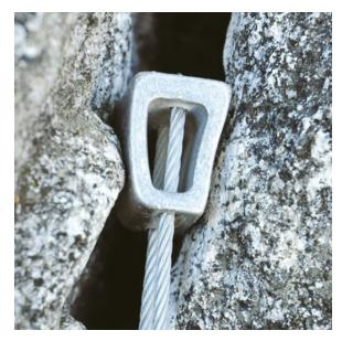
Marginal. This Stopper is in a good bottleneck, but since it lacks flush contact on the right side, a slightly outward pull will pluck it from its placement.
