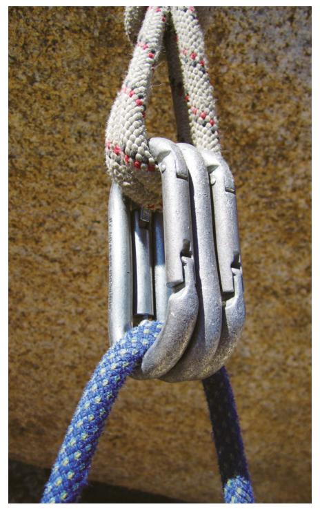
Three steel ovals with the gates opposed and reversed at a toprope anchor.
