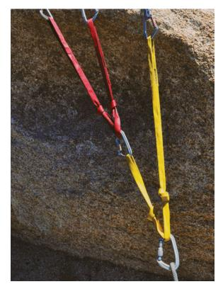
Here the rigging is redundant with minimal extension. The two pieces on the left have been equalized with the red 48-inch nylon sling, using a sliding X and extension-limiting overhand knots. The yellow 48-inch nylon sling equalizes this point to the single, strongest piece in the anchor, again with a sliding X and extensionlimiting overhand knots.
