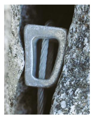
Stopper in a bottleneck placement. There is simply no way that in a downward pull the nut could be pulled through the bottleneck something would have to give, either the rock itself or the nut or wire cable breaking.
