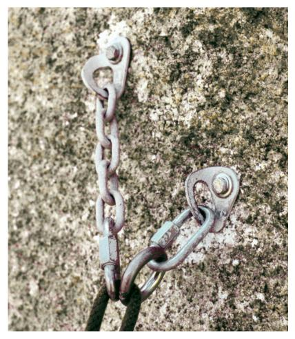
A well-engineered rappel anchor. Both bolts are ¾-inch stainless Powers bolts with stainless steel Petzl hangers, along with a stainless steel chain, quick link, and ring. Everything was painted before installation to match the color of the rock.
