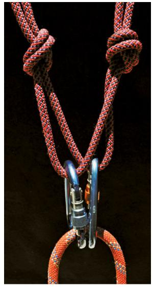
Detail of the equalette master point using two locking carabiners opposed and reversed.
