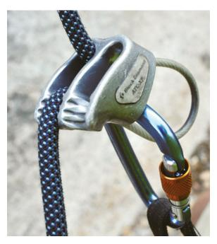
Black Diamond ATC XP in high-friction mode with the teeth on the braking side.
