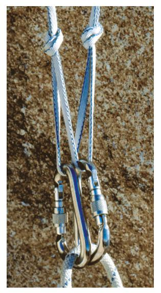
Detail of equalette master point rigged with a Dyneema sling. Tying an overhand knot in a Dyneema sling reduces its strength by 50 percent; it's better to use a 7mm nylon cordelette when rigging the equalette, as you'll be tying lots of knots.
