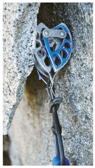
This camming device has been placed behind a flake of rock (left). If the cam is loaded, it will pry outward, potentially breaking the flake. This can cause the anchor to fail and also send the chunk of rock tumbling down onto people below.
