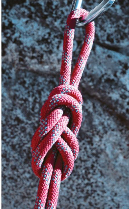
Finished figure eight loop clipped to an anchor.
