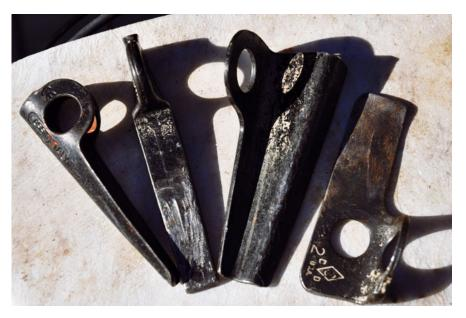
*Pitons (left to right): Angle, horizontal, Leeper Z, knifeblade.*
