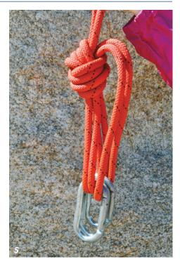
4 & 5 For greater security, take the single loop and hitch it all the way back around the body of the two-loop knot or clip it into the carabiners on the master point.
