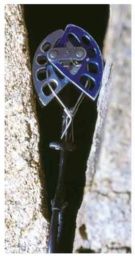
Bad. Even though the cams on this Black Diamond Camalot are within the acceptable range (right around 50 percent retracted), the widening crack above will allow the cams to easily "walk" into the wider section, even with minimal loading and unloading of the device. Avoid this situation, since the cams can potentially walk to an open and unstable position.
