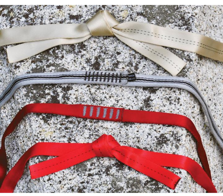
Nylon Webbing Comparison. Top to bottom: 1-inch tubular nylon webbing tied with water knot (Sterling Tech Tape, rated at 4,300 lbs. tensile strength); 18mm Metolius Nylon Sling, rated at 22 kN loop strength (4,946 lbs.); 18mm Black Diamond Runner, rated at 22 kN loop strength; <sup>11</sup>/<sub>16</sub>-inch Sterling tubular webbing tied with a water knot (rated at 3,000 lbs. tensile strength).
