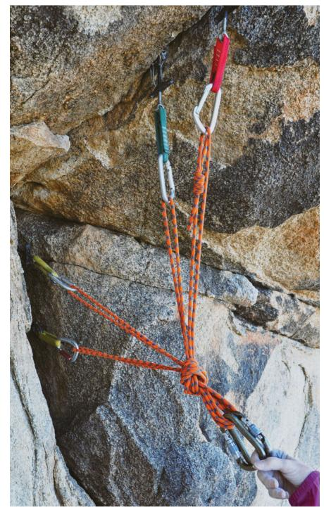
Four-piece uniform load anchor pre-equalized with a cordelette in the anticipated direction of load. If the load shifts even slightly, all of the *load will come to bear* on a single piece. If that piece were to fail, the vector would shift to the next piece to load, albeit with minimal extension from the cordelette. The cordelette system is essentially a series of backups rigged with minimal extension.
