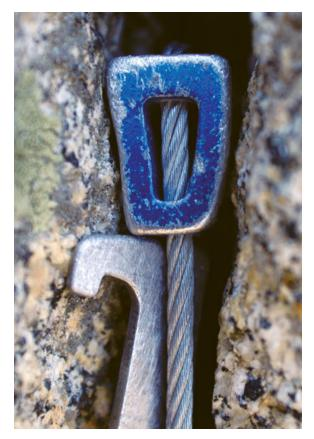
To remove a nut with a nut tool, inspect the placement and determine the intended direction of pull, then tap in the opposite direction.
