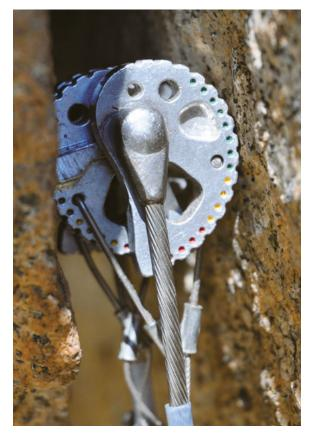
Good. This Metolius Power Cam displays optimal green "range finder" dots in a solid, parallel-sided crack.
