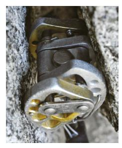
Fair. This Camalot is in a slightly flaring crack, with the inside cams retracted tighter than the outside ones, although each set of cams (inside and outside) are within a suitable range and all the cams have flush contact with the rock.
