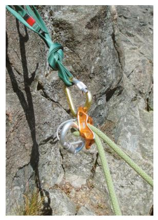
An autoblocking device set up in "guide mode," loaded with the climber strand on the top and the belay strand on the bottom.
