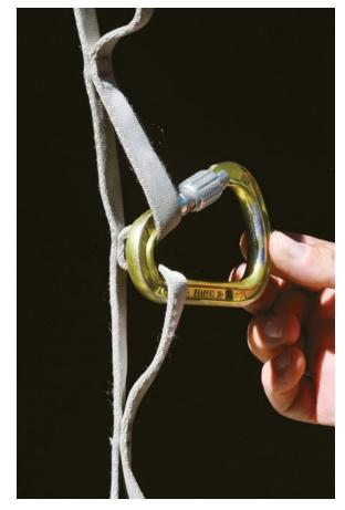
A traditional daisy chain with bartacked pockets is not recommended for rappel extensions or as a personal tether, because if a carabiner is clipped into two loops, an extremely weak connection is created (3 kN or 674 lbs.).
