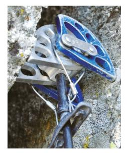
Very poor. The cams are barely retracted and nowhere near the recommended range. The piece can easily walk and might fail completely.
