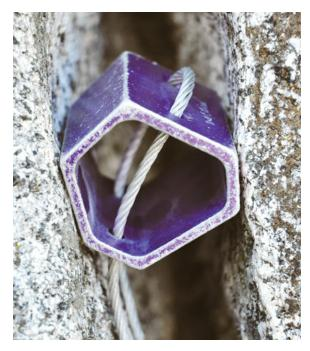
Good. This Hex is in a narrowing pocket, and both sides of the nut have good surface contact.
