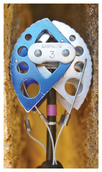
Very good placement. All the cams have good surface contact in a solid, straight-in crack, and the cams are in the recommended range for a Camalot (50 to 90 percent retraction).
