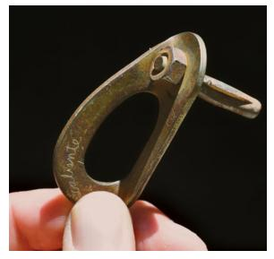
The infamous <sup>1</sup>/<sub>4</sub>-inch threaded Rawl Drive contraction bolt, complete with the SMC "death hanger." This ticking time bomb was removed and replaced from a route on Suicide Rock, California.
