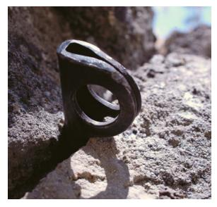
An angle piton, driven all the way to the eye—a good placement.
