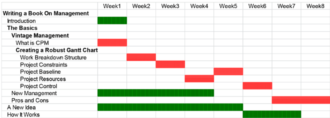
Figure 2-2. Gantt chart representation of an earlier WBS with an emphasis on time
