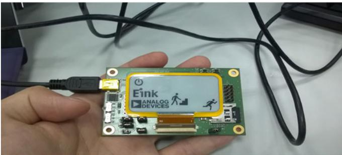
Fig. 4 ADXL362Z-DB triaxial accelerometer
