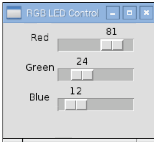
Figure 14-14. Adjusting the RGB LED Color Using a User Interface
