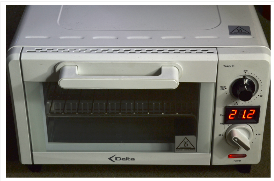
Figure 20-21. A Homemade Reflow Oven
