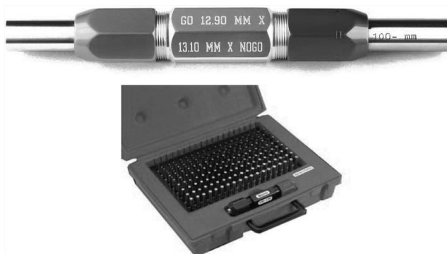
FIGURE 28.2 Typical pin gage and set of pins.
