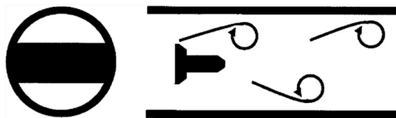
FIGURE 58.2 Vortex shedding in a pipe.
