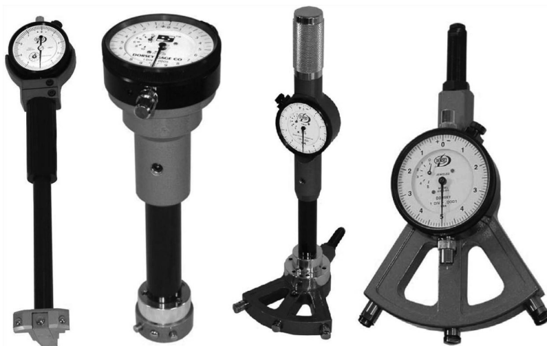
FIGURE 28.9 Multipoint contact bore gages.
