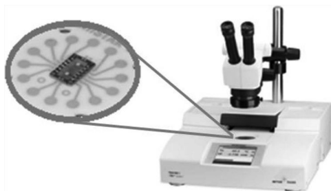
FIGURE 79.2 Flash DSC 1 of Mettler-Toledo with a close-up of the device UFS 1. The device is made of two identical cells, the reference and the sample cell, respectively. Both cells consist of two heaters covered with an aluminum layer that makes up the sample area, in the center of the membrane; the hot junctions of the eight thermocouples are inside the sample area.
