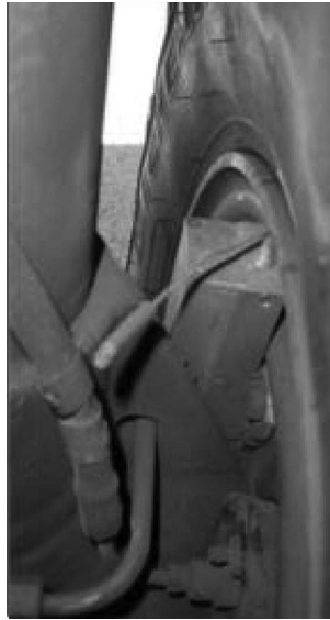
FIGURE 87.2 Ruggedized wireless wheel vibration and temperature sensor. (Courtesy of Solidica, Inc., Ann Arbor, MI.)
