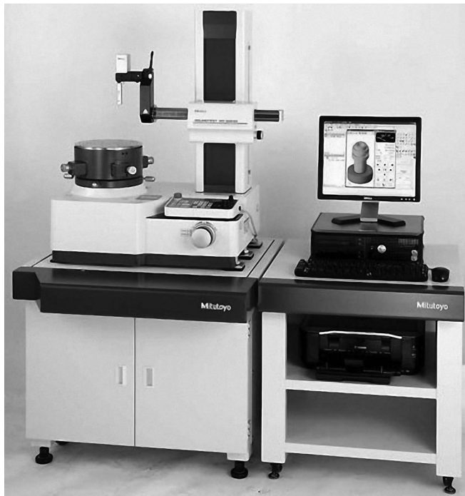
FIGURE 28.14 Round test RA-2200AS/DS/AH/DH by Mitutoyo.
