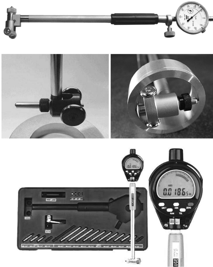
FIGURE 28.4 Self-centering two-point bore gage.
