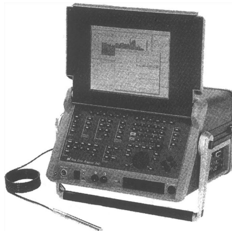
FIGURE 48.11 Real-time frequency analyzer for acoustic measurements.
