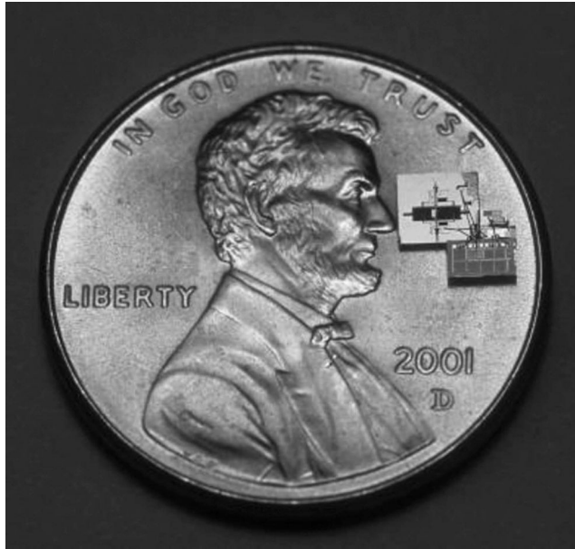
FIGURE 86.1 Smart dust sensor node that includes optical communication, sensors, and power. Approximately the size of a grain of rice.
