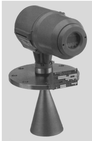
FIGURE 18.8 Design of a compact industrial level RADAR system. The converter above the flange includes the complete microwave circuitry, signal-processing stages, microprocessor control, display, power supply, and output signal. (From Messtechnik, K., Technical Data Sheets of Level Measurement Products , Krohne, Duisburg, Germany, 1996.)
