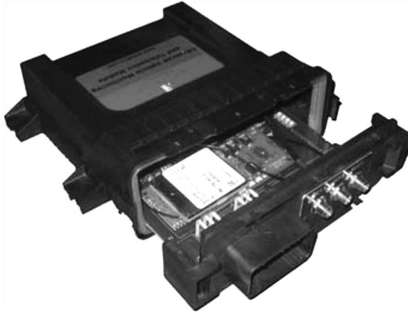
FIGURE 87.4 Commercially available EVAN device with J1979, J1708, J1939, GPS, cellular, 802.15.4, and 802.11b/g capability. (Courtesy of Solidica, Inc., Ann Arbor, MI.)
