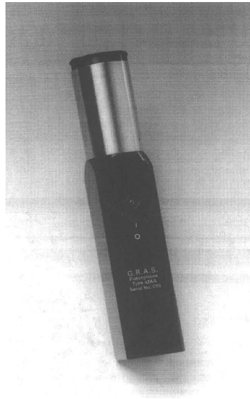
FIGURE 48.20 Pistonphone for microphone calibration.
