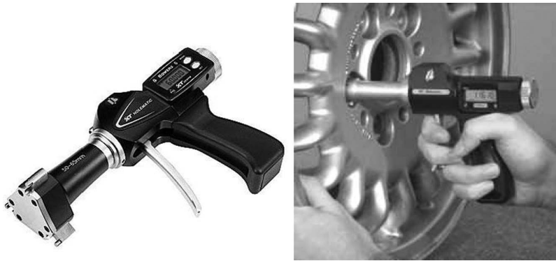
FIGURE 28.8 Pistol-grip bore gage and its use.
