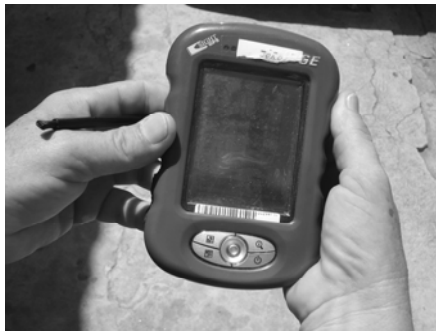
Fig. 3. Field use observation: the device under the sunlight has legibility impaired
