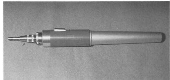
Photo 17. Battery-operated tool for graft removal by power punch
