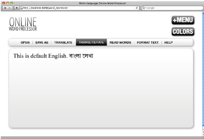
Fig. 2. Screenshot of the word processor, showing the basic functionalities and the transliteration enabled ( button in black background )
