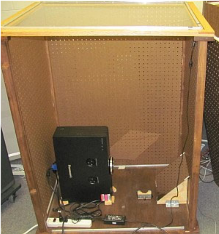
Fig. 1. A side view of the open MET displaying its internal components, including the projector, wiring and power sources, and mirror
