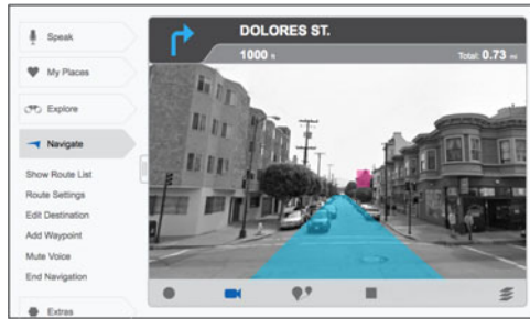
Fig. 4. Navigation tool that uses the device's viewfinder as the primary interface and enhances it with a wealth of contextually relevant information
