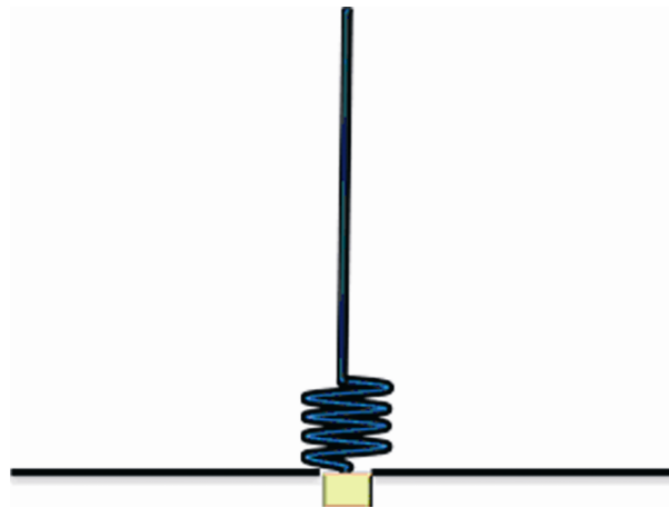
Figure 9.11. Monopole loaded by inductor (whip monopole)
