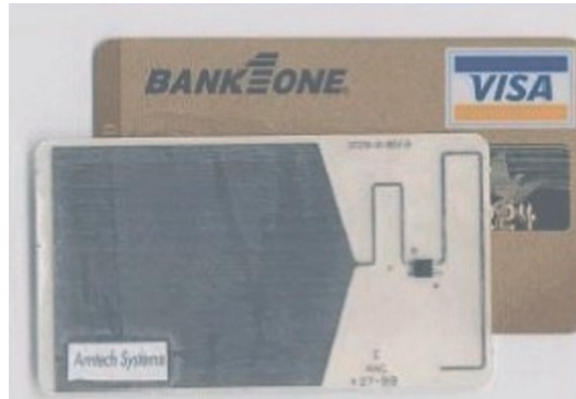
Figure 1.4. Meander line dipole antenna for use in RFID applications
