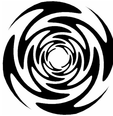
Figure 8.8. Dual polarized sinuous antenna
