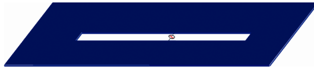
Figure 9.4. Structure of a slot antenna
