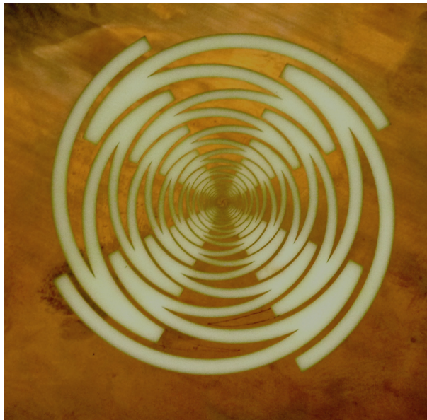
Figure 8.10. Modified dual polarized sinusoidal antenna
