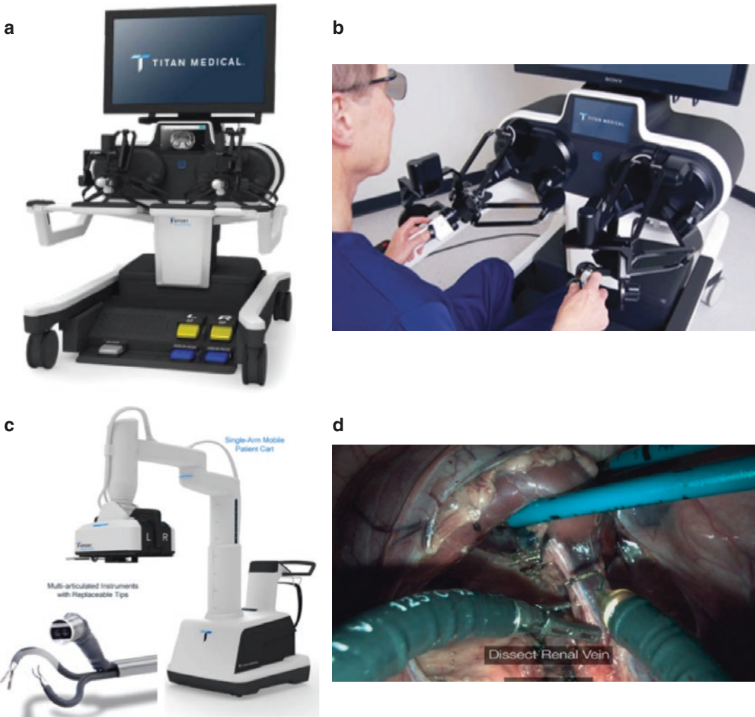
Fig. 1.15 SPORT™ Surgical System (Titan Medical, Canada) for robotic single-port surgery. (a) Console offering 3D–HD–vision, armrest, two handles, and foot-pedal to control monopolar and bipolar cautery. (b) Transfer of movements at the console with sigma-technology (Force Dimensions, Nyon, Switzerland). (c) Robotic arm to
