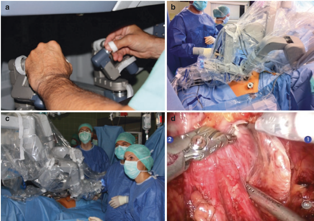
Fig. 1.5 Da Vinci S—next step of robotic evolution. (a) Unchanged basic console design, but with integrated bipolar foot pedal, optionally HD-camera and fourth arm-pedal). (b) New robotic arms (three or four) with wider
