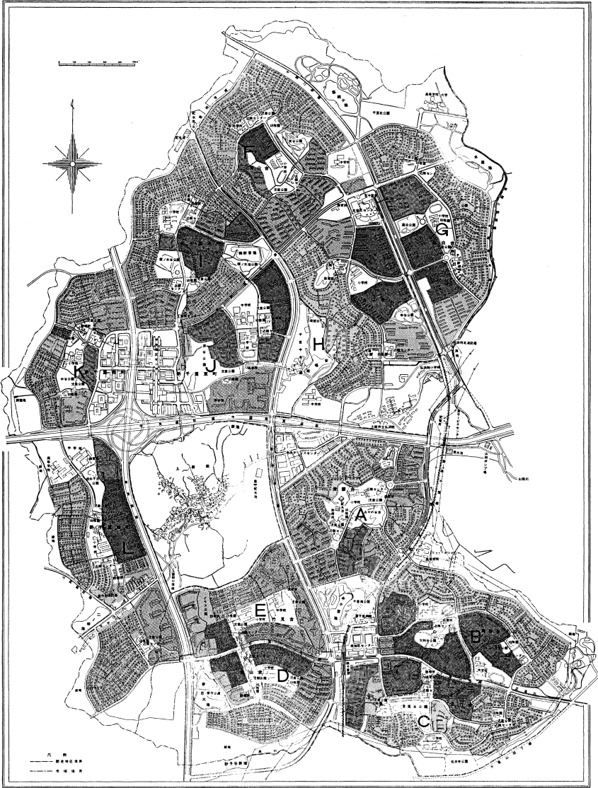
Figure 5.11 Senri New Town Master Plan. Senri, north of Osaka, is typical of the “New Towns” which started to appear in the mid-1960s. While still primarily designed to supply large volumes of new housing, Senri also included a town centre, expressway grid, rail stations, and recreation facilities.
