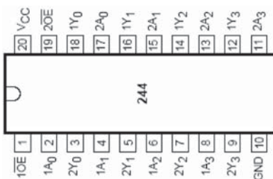
FIGURE 10.12. Line driver used with external LEDs to display the spectrum in project graphic_FFT .
