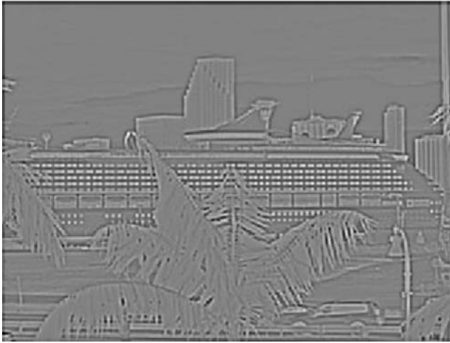
FIGURE 13.30 Image edge detection using Laplacian of Gaussian filter.
