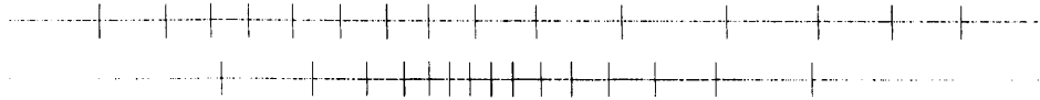
Figure 19.7: Quantization thresholds found by the scalar quantization algorithm for uniform and Gaussian distributed data. For both cases 1000 points were generated, and 16 centers found by running the basic scalar quantization algorithm until convergence.
