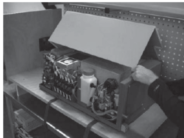
Figure 14.32 (a) Fuel processor of the VeGA system [16]. (Source: O'Connell et al. [16]. Reproduced with permission of Elsevier.) (b) 250 W el fuel cell/fuel processor system VeGA developed by a cooperation of TRUMA and IMM [106]. (Source: Wichert et al. [106]. Reproduced with permission of Elsevier.)
