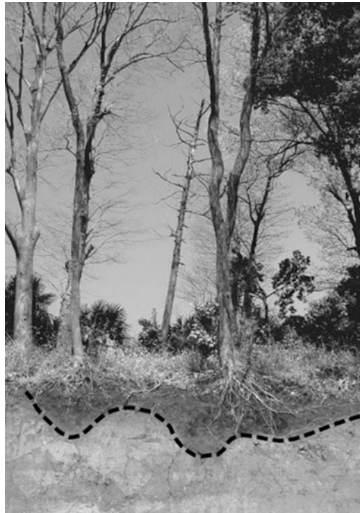
Fig. 3.2 Results of dye tracer experiment demonstrating (a) fingering (modified from Iida and Hamada 2009) and (b) macropore flow (after Scanlon et al. 1997)
