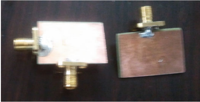
Fig. 12.52 Top and side view of single- and double-feed aperture couple feed of RDRA
