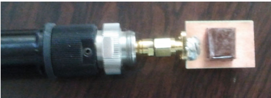
Fig. 12.60 Fabricated model of RDRA under test with single feed and slot
