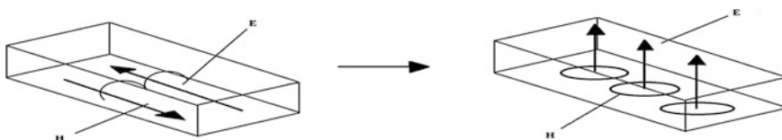
Fig. 7.3 EH fields pattern or resonant modes
