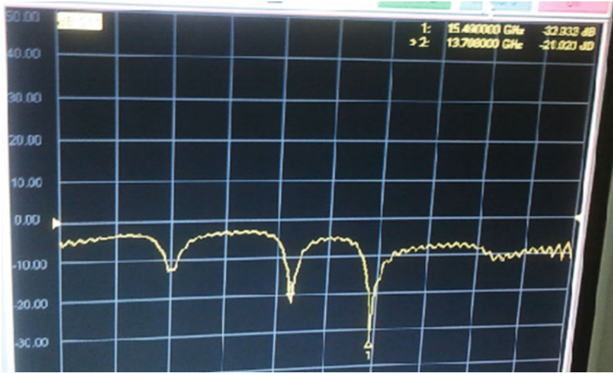
Fig. 12.59 VNA showing measured S11 of RDRA
