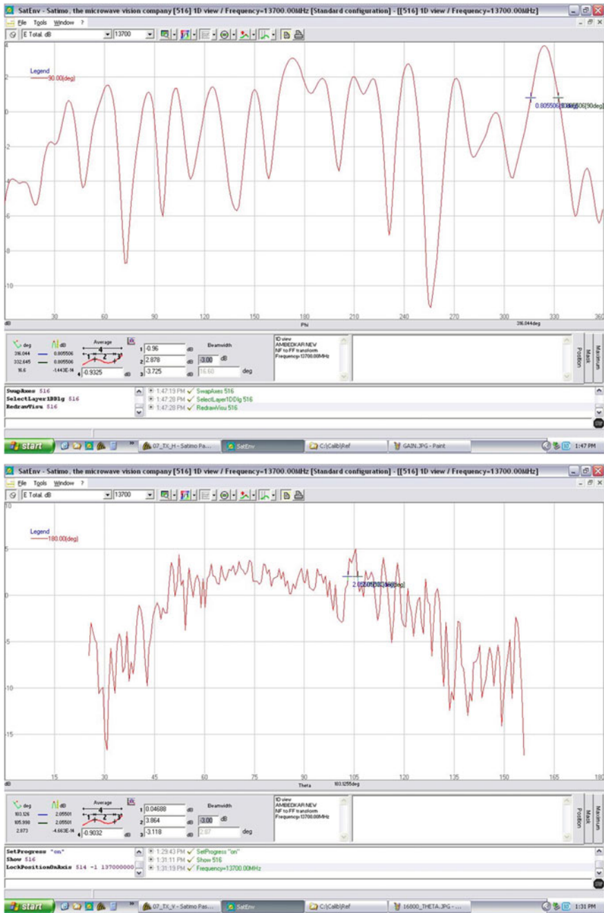
Fig. 12.13 Radiation pattern at 13.7 GHz for radiated field pattern of simulated RDRA
