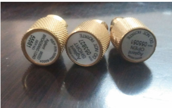
Fig. 12.51 Short, open, and load termination for calibration of VNA
