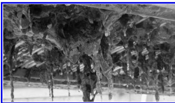
FIGURE 5.35 Fibrous materials can block the air-liquid channel, if screen fails regardless of membrane types. (Courtesy of Mott MacDonald.)
