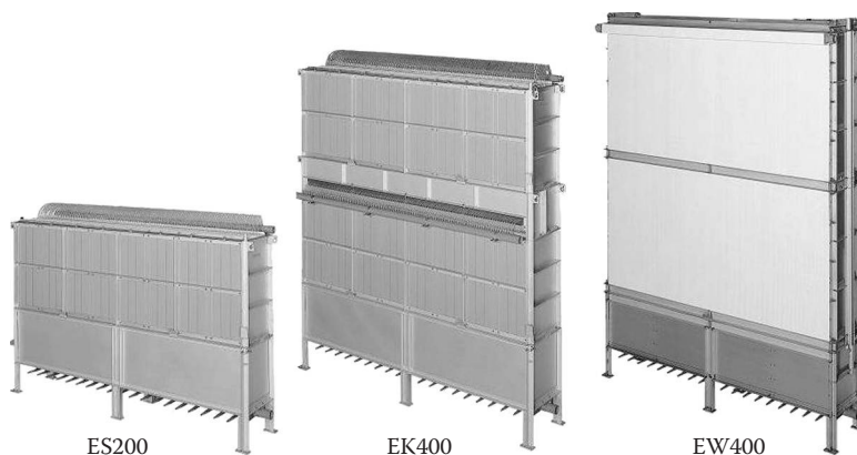
FIGURE 2.21 Various types of submerged membrane unit (SMU) equipped with flat sheet membrane panels: ES200 (0.8 m 2 × 200 ea., 2.0 m high), EK400 (0.8 m 2 × 400 ea., 3.5 m high), and RW400 (1.45 m 2 × 400 ea., 4.3 m high). (Courtesy of Kubota Membrane USA Corporation.)
