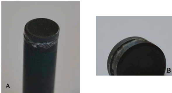
Figure 1. Braze SiC specimens: (A) tube and lid; (B) disks.
