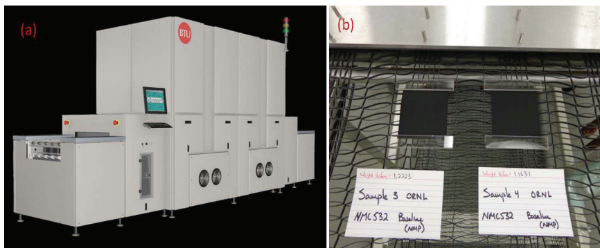
Figure 3: (a) BTU's inline MW system (b) Electrodes entering into the MW exposure zone
