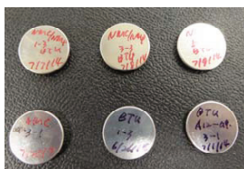
Figure 4: Coin cells prepared using microwave dried electrodes
